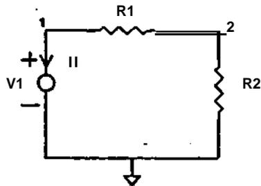
Using MNA, three equations are written to solve this circuit. Two of the equations will add the currents leaving each of the nodes. The third equation will specify the branch relation of the voltage source. The equations resulting from an MNA analysis of the circuit are:
