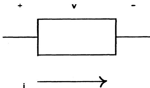
That is, current always flows from the positive to the negative terminal of an element. In addition, the ASP convention is that the positive terminal is always defined first. Be especially careful of this when defining current sources.
