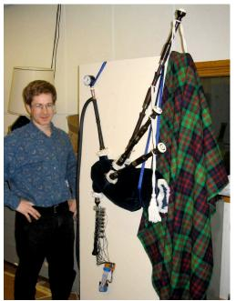
Figure 4. Garth Zeglin with McBlare shortly before its debut at the Robotics Institute's Twenty-Fifth Annivesary. Bagpipes are mounted on a display board that conceals the pump and additional electronics.
