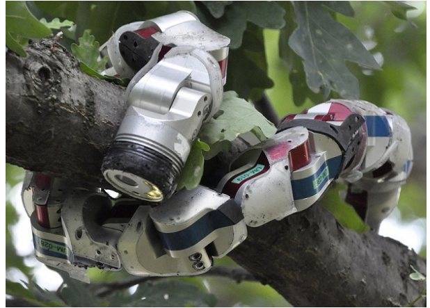
Fig. 1: Photograph of the Unified Snake Robot climbing a tree.
