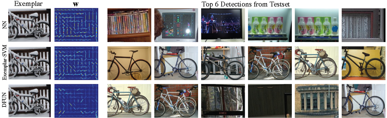
Figure 3. Comparison. Given a bicycle training sample from PASCAL (represented with a HOG weight vector \mathbf{w} ), we show the top 6 matches from the PASCAL test-set using three methods. Row 1: naive nearest neighbor (using raw normalized HOG). Row 2: Trained Exemplar-SVM (notice how \mathbf{w} focuses on bike-specific edges). Row 3: Learned distance function – an Exemplar-SVM but trained in the “distance-to-exemplar” vector space, with the exemplar being placed at the origin (loosely corresponding to [10, 14]).
