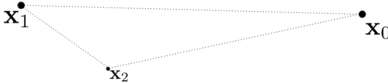
Figure 4.5: Geometric condition to control information leakage. When we compare two transformed points against a third transformed point, the information leakage is negligible if this third point is far enough.
