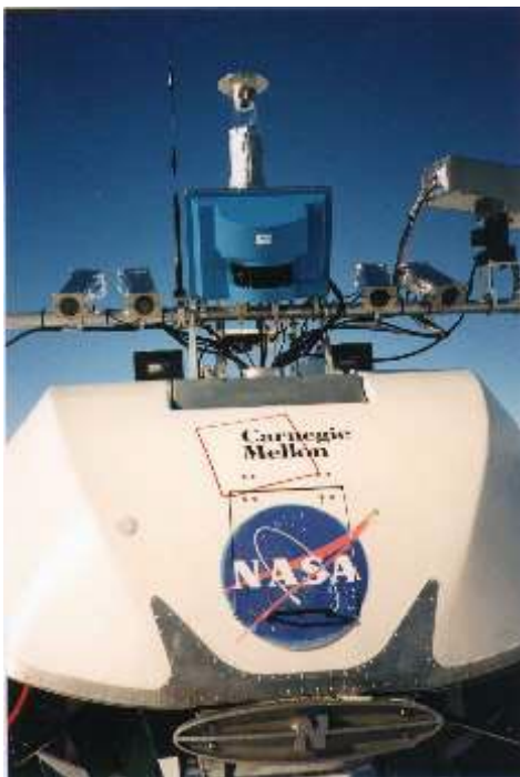
Figure 3: Nomad's sensor yard with 4 CCD cameras and SICK LMS 220 single line scan laser unit.
