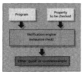
The verification process begins with a program (or a description of a circuit design) and a list of properties to be checked. The verification tool determines if the properties are true, or if not, provides a counterexample.
