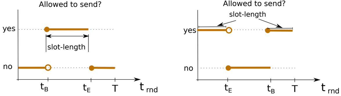
Figure 4.2: Defining a TDMA slot and respective boundaries. Left) Boundary  $t_B$  is less than  $t_E$ . Right) Boundary  $t_B$  is greater than  $t_E$ . Inside a slot, a node is allowed to transmit packets (cf. Equation 4.2). Slot length is also depicted (cf. Equation 4.3).
