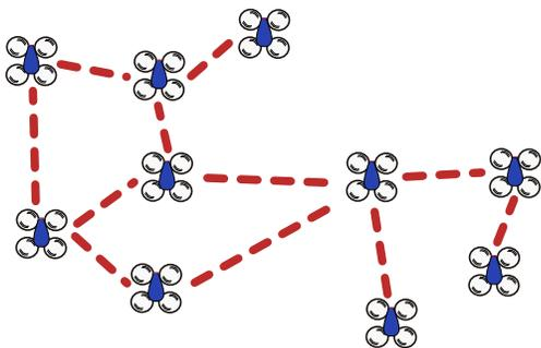
Figure 1.5: A quadrotor swarm and communication links (red dashed-lines).
