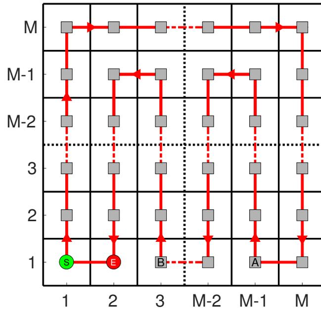
Figure 7.4: Square AoI with even number of cells to visit ( $M^2$ ). Side size is  $W$ . Red path describes the shortest tour, and it starts at "S", it ends at "E", and restarts at "S" again. Tour length  $d$  is optimal and equal to  $d_{\min}$ .
