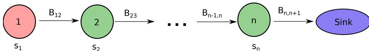
Figure 5.1: Multi-hop Line Network model. Bandwidth of each link is represented by  $B_{i,j}$ . Variable  $s_i$  represents the units of time (time slot) available to each node to transmit periodically every  $T$ .
