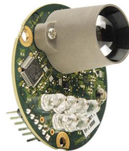
Figure 1.6: LeddarOne is a LIDAR sensor designed for small UAVs.
