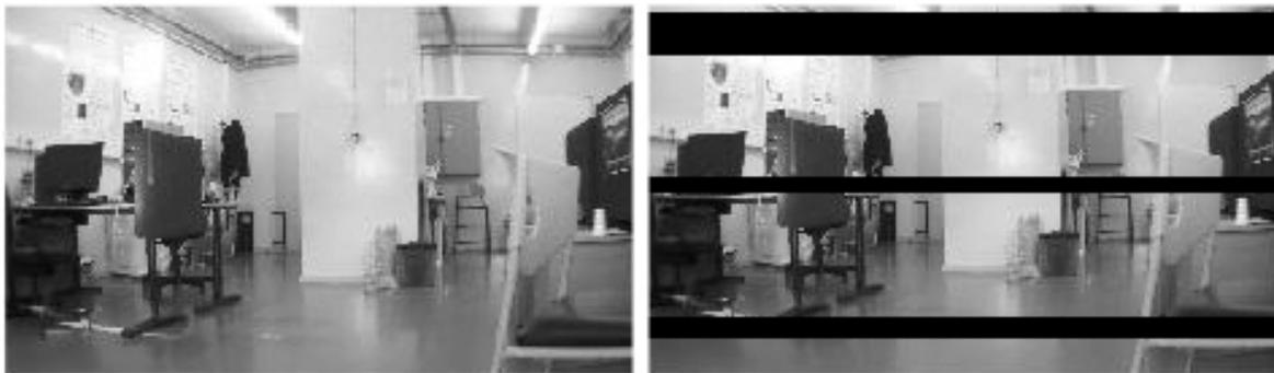
Figure 5.15: Snapshot of the video stream at the sink. With CSMA/CA (on the right), relays cannot handle every received packet, dropping some that appear as black lines in the image. Under DVSP (on the left), video streaming is visibly improved and frames are generally complete.
