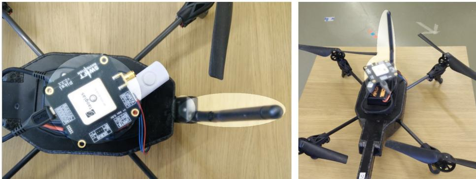
Figure 8.3: Piksi GPS on a drone – This unit is mobile and receives data from the fixed GPS unit via dedicated radio, which can be seen in Figure 8.2.
