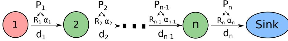
Figure 6.1: Multi-hop line network model. The PDR of link  $i$ , between nodes  $i$  and  $i+1$ , is  $P_i$  with parameters  $R_i, \alpha_i$ , and its length is  $d_i$ .
