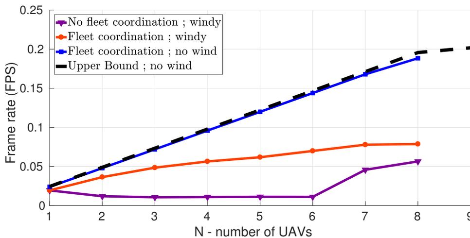
Figure 7.8: Maximum global frame rate to sweep the AoI, with wind gusts pointing north at 6m/s with and without our formation algorithm in place. AoI:  $L = 20\text{m}$ ,  $M = 4$ ,  $C_{GS} = 323\text{kbit/s}$
