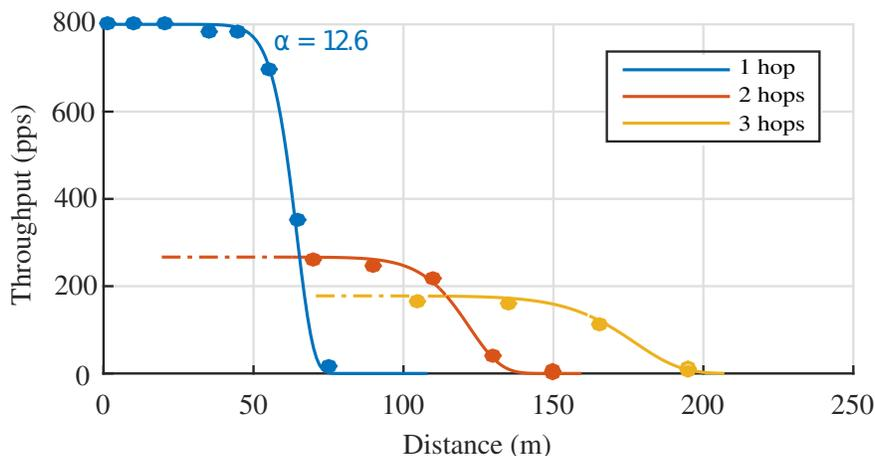
Figure 3.6: Measured throughput at different end-to-end network lengths, using distinct number of hops. Inside their slots, nodes transmit 200-byte packets at a rate of  $B \approx 800$  pkts/s. UAVs are all oriented parallel to each other.
