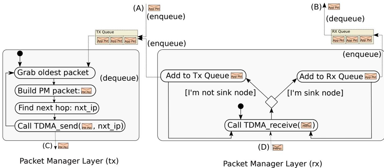
Figure 8.5: Packet Manager (PM) layer, routes packets to the next hop, or holds them for the AL if packets have reached their final destination (Sink). Communicates both with AL (above) and TDMA layers (below).
