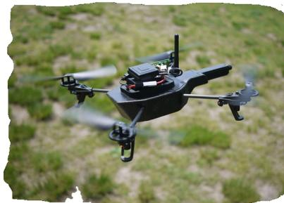
Figure 3.1: AR Drone 2.0 platform, a common COTS quadrotor, used for the experiments.
