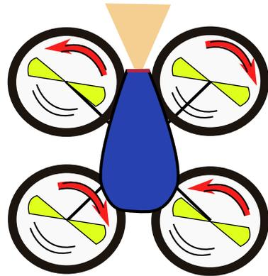
Figure 2.1: Drone with four rotors. Propellers rotate in different directions to counteract angular acceleration.
