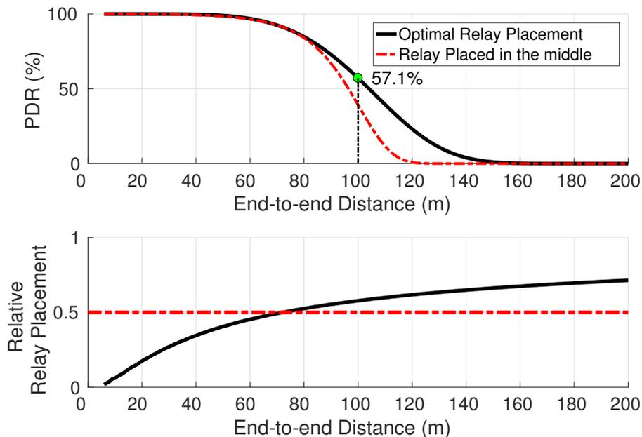
Figure 6.4: (top) End-to-end PDR on a two-link network as a function of end-to-end network length  $L$  (links modeled as in Figure 6.3). (bottom) Optimal position of the relay as fraction of  $L$  (bold curve).
