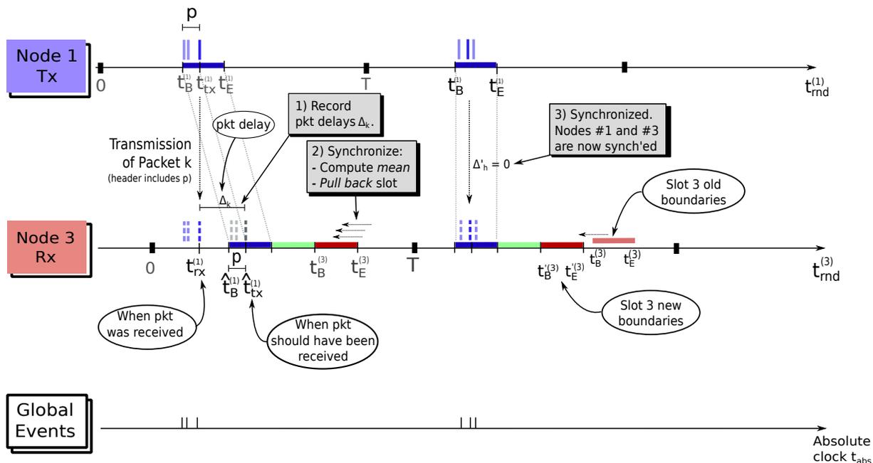
Figure 4.4: Illustration of TDMA self-synchronization mechanism taking place.
