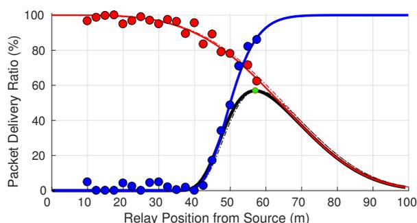
Figure 6.8: DRP final state. Relay estimated the optimal location at 57.8m from the Source.
