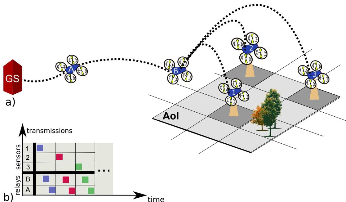
Figure 7.3: The network model encompasses: a) a multi-hop backbone of relay-UAVs that connects the sensor-UAVs (in the AoI)t to the GS; b) a TDMA network access scheme that grants one slot to each sensor-UAV for its exclusive use.
