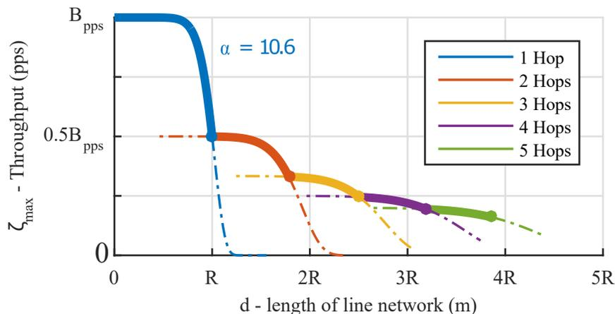
Figure 3.4: Maximum network throughput as function of distance –  $\zeta_{\max}(d)$ , in packets per second. Each colour represents a different number of hops in use in the network, described by a different section of Equation 3.17. Number of hops  $h \in [1, \dots, 5]$ , and updated at certain distances given by Equation 3.18. Link PDR assumes  $\alpha = 10.6$ .
