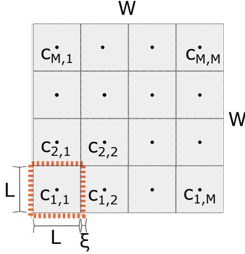
Figure 7.2: Square Area of Interest (side  $W \times W$ , and respective division into  $M \times M$  square cells.  $L$  is chosen such that if a vehicle is at the centre of a cell ( $c_{ij}$ ), with a maximum error of  $\xi$  in any direction, then the cell is fully contained in the field of view of a UAV.
