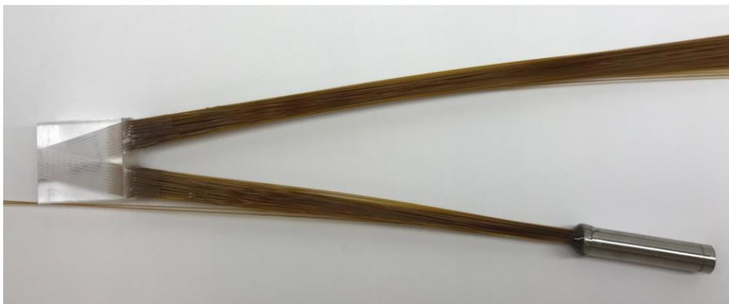
**Figure 2.10.** The photograph of the microreactor after 100 inlet and 100 outlet capillaries are glued in to the block and stainless steel inlet flow divider is prepared.
