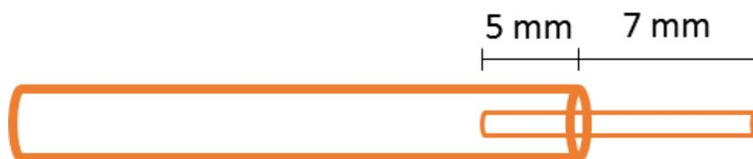
**Figure 2.9.** The schematic representation of the gluing process for the preparation of quartz capillaries that will be guiding flow to and from the microreactor.
