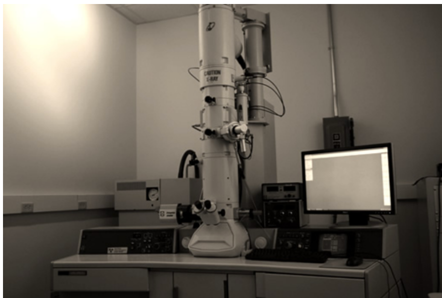
Figure 3- 1 JEOL JEM-2000EX Transmission Electron Microscope
