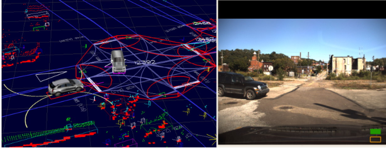
Figure 4.24: The autonomous vehicle stops at a four-way-stop intersection, and waits for its turn to move
