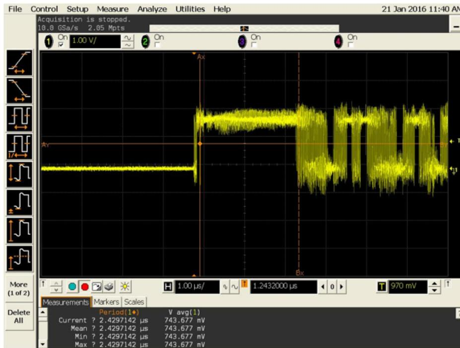
Fig. 4.20: The output voltage of a single neuron of the PLL ONN.
