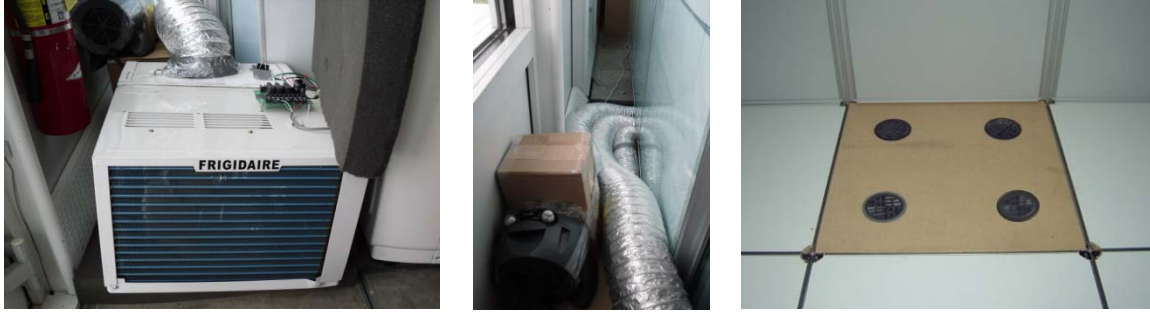
Fig. 24. Air conditioner and two portable heaters are connected through flexible ducts to the floor diffusers of the chamber
