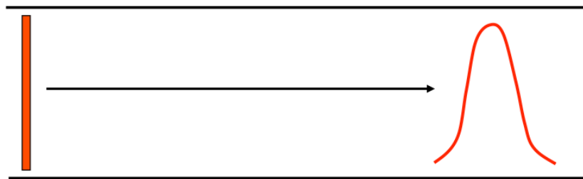
Figure 2.1. Cartoon showing the band broadening of a pulse injection in a packed bed column.
