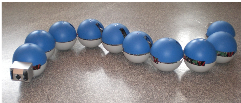
Figure 6.4: The Kulko robot from NTNU. This robot has spherical housing and force sensing resistors in each link, and performs obstacle-aided locomotion by controlling the contact forces along its body. Printed with permission of the authors of [57].
