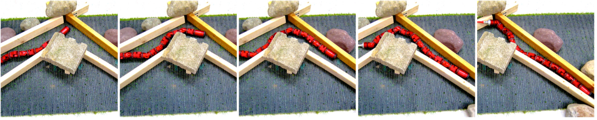
Figure 9.6: A montage of the robot undergoing the a low-impedance slithering gait. The robot executes the gait cycle and progress forward, but can be easily deformed form the nominal shape. This allows the robot to progress around a bend that would not have been possible with a standard position-controlled gait.
