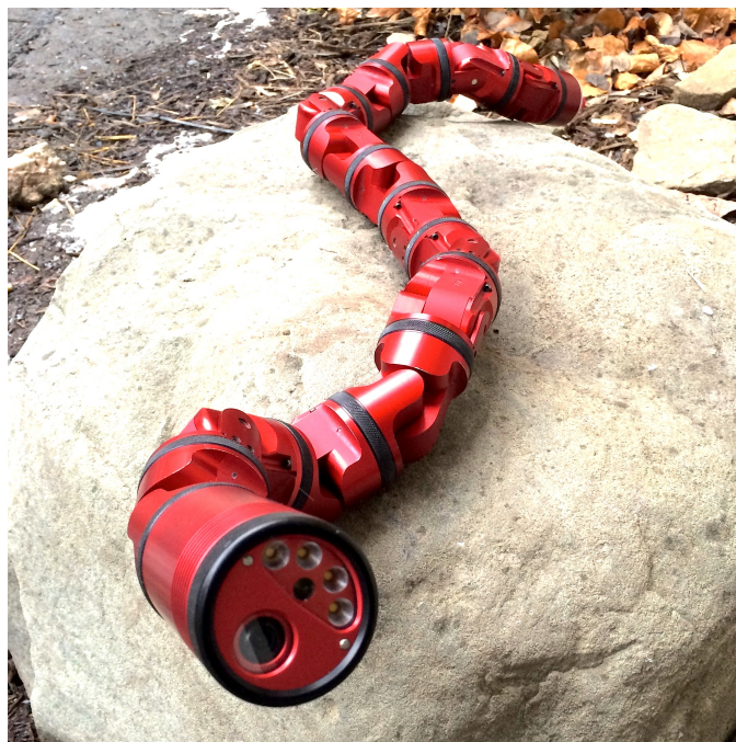
Figure 8.1: A photo of the Series Elastic Actuated Snake robot ( SEA Snake ). Each module of the robot has series elastic actuation that enables compliant motion and torque sensing.
