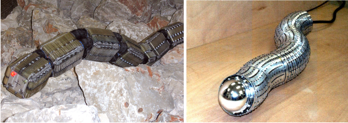
Figure 6.3: Examples of compliantly actuated snake robots. The OmniTread OT-4 robot (left) has rigid tracked sections joined by pneumatic bellows. The Slim Slime robot (right) is a continuum robot with internal pneumatic actuators. Presented, respectively, with permission of the Prof. Johann Borenstein and Prof. Shigeo Hirose.
