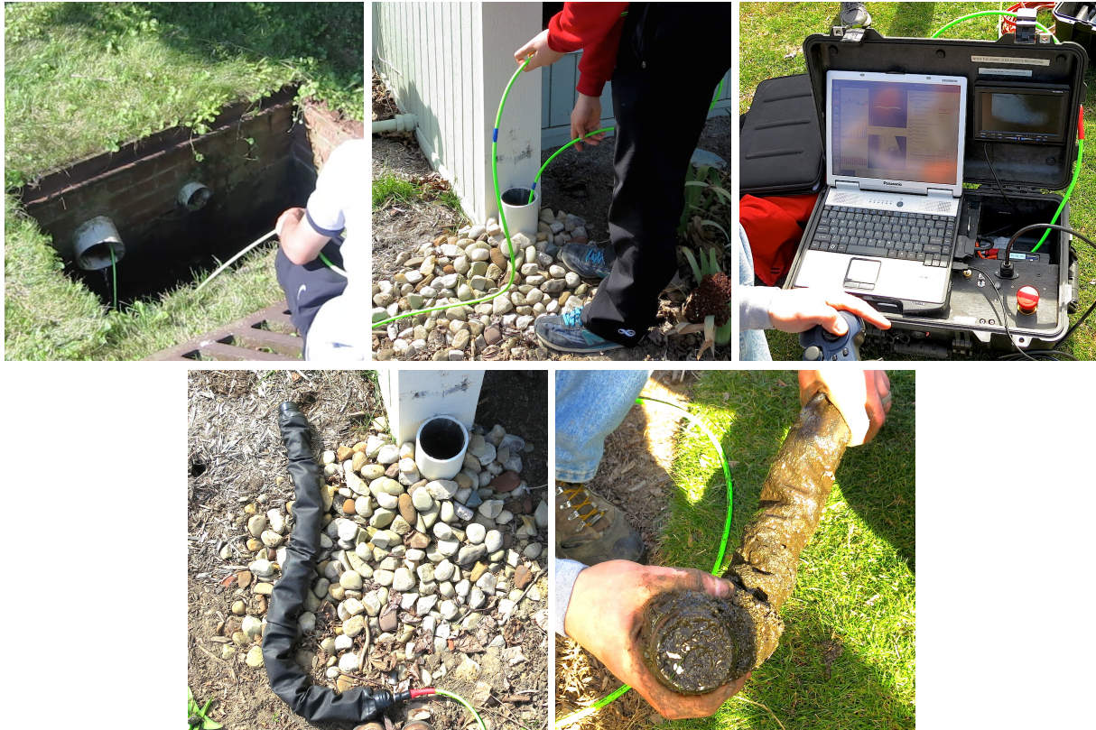
Figure 5.10: Photos from the field deployment of the snake robot. The top images show the two locations where the robot was inserted into the storm sewer and the operator control unit. The bottom images show the robot before deployment (left) and after retrieval from the storm sewer (right).
