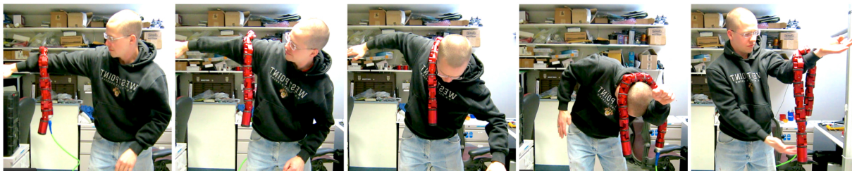
Figure 9.2: A montage of the robot undergoing the compliant roll-in-shape motion. The robot actively rolls along while compliantly adapting its shape to match its surroundings.
