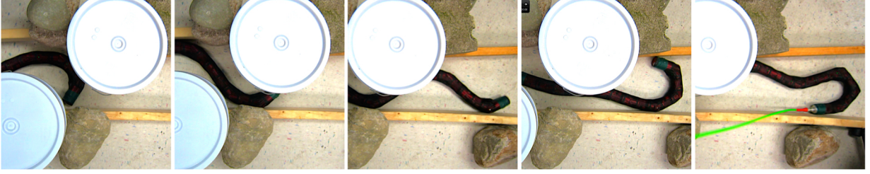
Figure 9.5: A montage of the low-impedance sliding motion. The robot’s head oscillates until the shape of the robot closely matches the shapes of the buckets and the snake slides through. Afterwards, the head continues to oscillate, causing the robot to turn in place.
