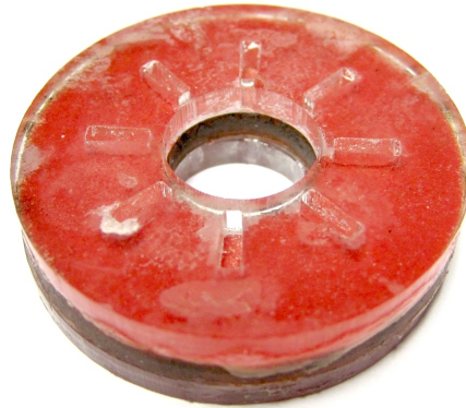
Figure 7.2: A photo of one of the early prototypes of the series elastic spring. The rubber element is latex sheet, which is glued to acrylic plates. The spring is 38 mm (1.5 in) in diameter and 10 mm (.4 in) thick.
