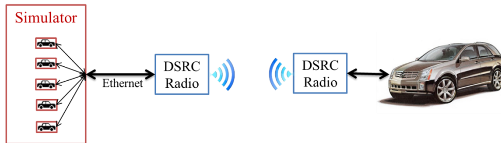
Figure 9-3: AutoSim: Interaction of Real and Simulate vehicles though DSRC.
