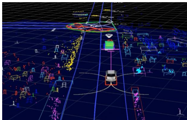
Figure 9-7: V2V Distance Keeping between the EHDV and the AV.
