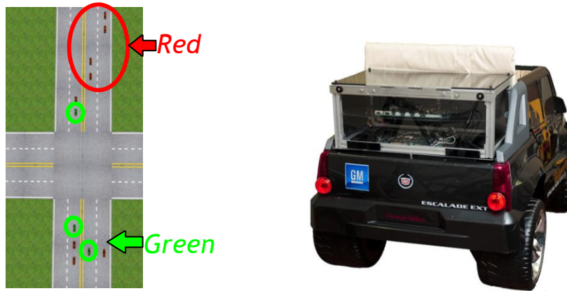
Figure 9-4: PowerWheels platform and Car-Following among real (green) and simulated (red) vehicles.
