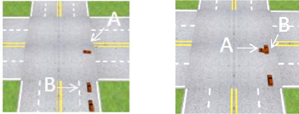
Figure 6-8: Snapshots from AutoSim simulator (a) No packet loss and safe passage of vehicles, (b) High packet loss rate results in an accident
