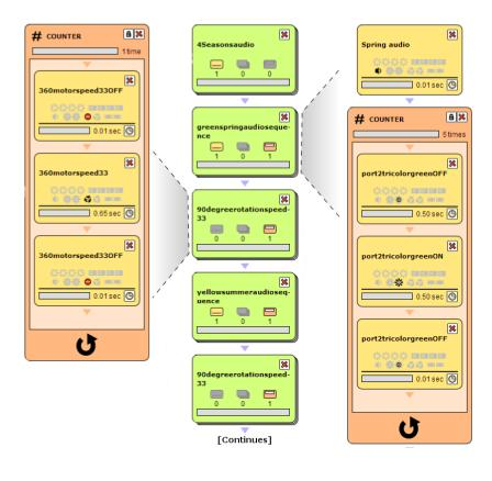
Figure 6.7: The main sequence created for the "Human Seasons" poem-bot is shown center. To either side are views of the contents of the subsequences; to the left is the subsequence for rotating the platform 90 degrees and to the right is the subsequence for the presentation of the Spring-Childhood stanza.
