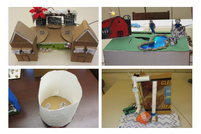
Figure 7.2: Four robots illustrating different degrees of Mechanical Sophistication, and Communication and Artistry: (clockwise from top left) audience consideration with direct motion; audience consideration with transformation mechanism; practical construction with transformation mechanism; practical construction with direct motion.
