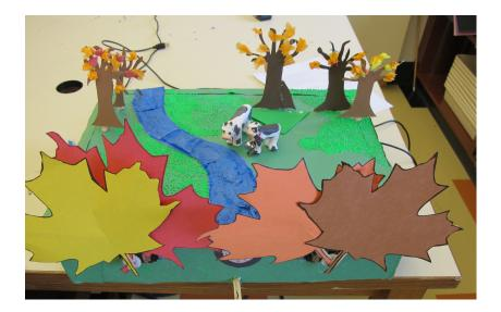
Figure 5.1: A poetry robot representing the poem "The Pasture" by Robert Frost that had trees and other components actuated by servo motors and LED lighting, which coordinated with a recorded reading of the poem.
