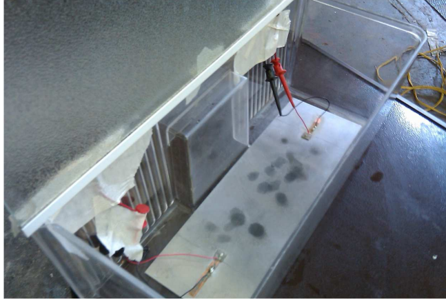
Figure 6.4: The experimental setup shows the aluminum plate and the two PZT (lead zirconate titanate) transducers used to monitor the plate.
