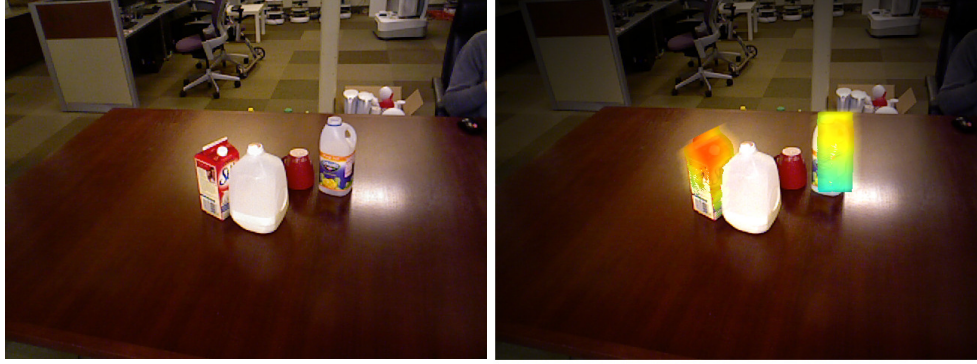
FIGURE 4.3: Example that demonstrates how C-PERCH can be used to obtain pose uncertainty estimates, including multimodal distributions. The object to be localized in this scene ( left ) is the milk carton (for which we have a 3D model) and the other objects are considered as extraneous clutter (no models available). C-PERCH yields two distinct solutions across multiple values of \alpha , which are overlaid on top of the input RGB image ( right ).
