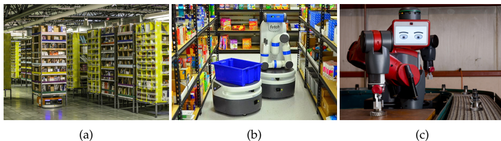
FIGURE 1.1: Examples of object instance detection tasks in warehouse automation and flexible manufacturing settings. (a) Amazon Kiva warehouse. (b) Fetch robot in an automated warehouse. (c) Baxter robot in a flexible manufacturing setup.
