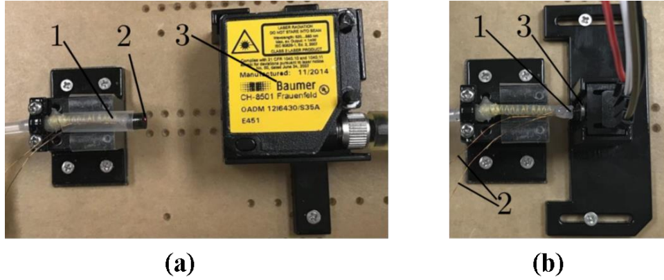
Figure 5.6: Sensors for characterization of the miniaturized actuation and sensing unit: (a) (1) soft actuator, (2) red laser beam point, (3) laser displacement sensor; (b) (1) soft sensor, (2) leads out of the soft sensor, (3) commercial force sensor.
