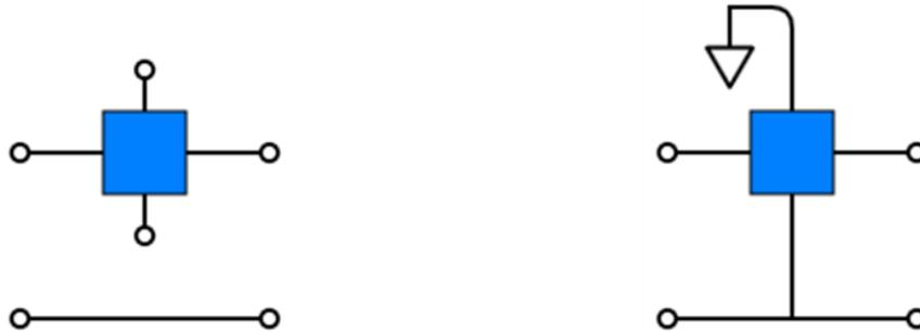
Figure 2.11 2P schematic showing the floating heater terminations (left) and grounded heater terminations (right) of the a series SPST implementation of an IPCS device
