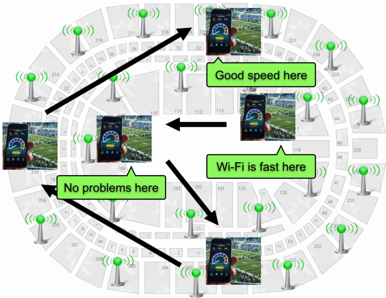
Figure 1.3: A typical site-survey procedure for a Wi-Fi network in a stadium. Wi-Fi engineers walk around the building while sampling Wi-Fi performance at various locations. The tools used often include Internet-speed-test mobile applications.
