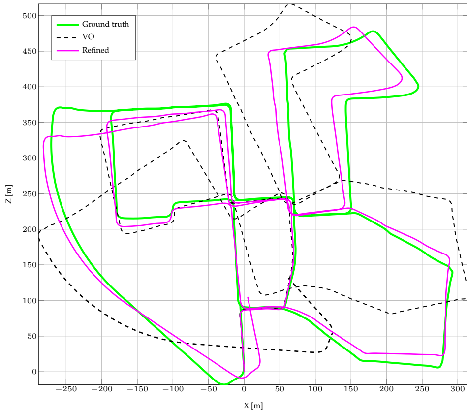
Figure 7.5: Magnitude of improvement starting from a poor initialization shown on the first sequence of the KITTI benchmark. Quantitative evaluation is shown in Fig. 7.4. We used a direct (correspondence-free) frame-frame VO method to initialize the pose parameters [15] (Chapter 6).
