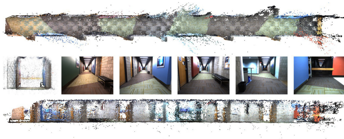
Figure 3.5: First row shows a top view from our indoor dataset. Images along the corridor are shown in the second row. The first image shows that floor of the model is flat as expected. The last row shows a side view of the corridor. The 3D points are obtained automatically from the algorithm without post-processing or filtering. The corridor length is \approx 40 m.
