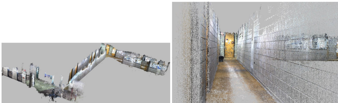
Figure 6.25: Reconstruction density using the Weal hall dataset Alismail et al. [11].
