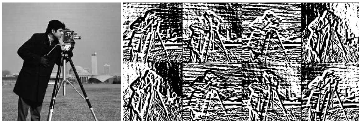
Figure 5.2: An example of the LBP descriptor evaluated on a 3 \times 3 neighborhood, which results in an 8-channel bit-planes descriptor.
