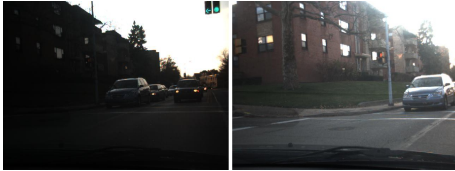
Figure 6.2: An example of the nonlinear intensity deformation caused by the automatic camera settings. A common problem with outdoor applications of robot vision.
