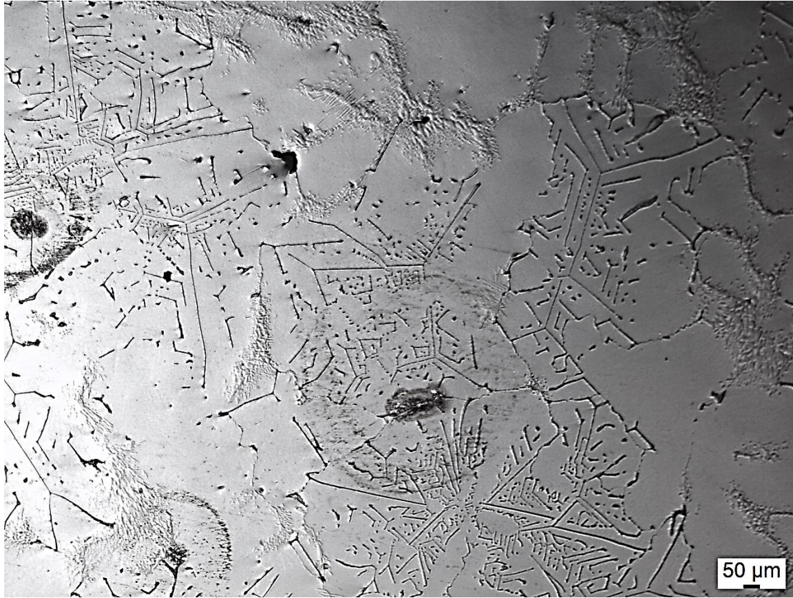
Figure C.5 OM micrograph of unetched Nb-modified tube UHCS microstructure. NbC structures and cementite/ M_7C_3 network are visible.
