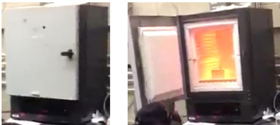
Figure A.1 Box furnace – open and closed.
