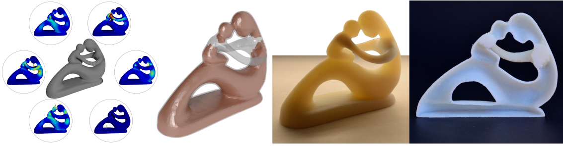
Figure 5.1: We present a method for lightweight structure design for scenarios where external forces may contact an object at a multitude of locations that are unknown a priori. For a given surface mesh (grey), we design the interior material distribution such that the final object can withstand all external force combinations capped by a budget. The red volume represents the carved out material, while the remaining solid is shown in clear. Notice the dark material concentration on the fragile regions of the optimum result in the backlit image. The cut-out shows the corresponding interior structure of the 3D printed optimum.
