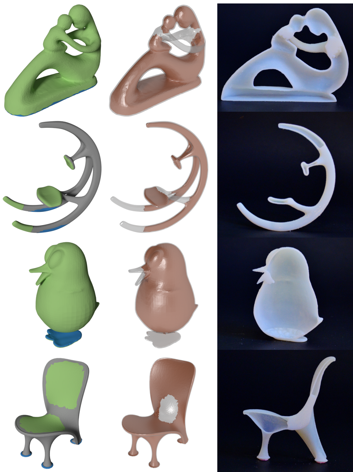
Figure 5.13: Structural optimization results. Left-to-right, problem setups with fixed boundary conditions (blue) and contact regions (green), our optimized structures and 3D printed cut-outs of optimal results. Red shows the removed material.
