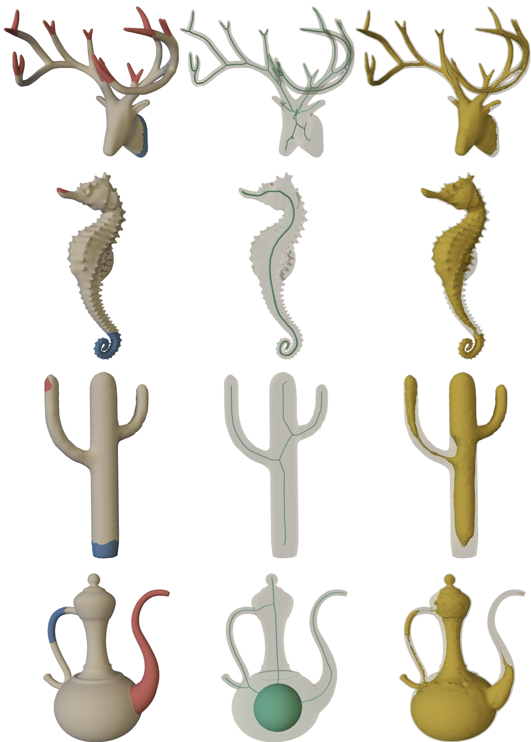
Figure 6.6: Structural optimization results. Left-to-right, problem setups with fixed boundary conditions (blue) and contact regions (red), skeleton structures used during the optimization and our optimized shell structures. Yellow shows the removed material.
