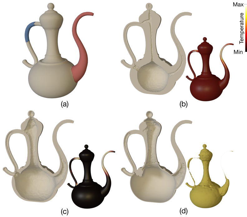
Figure 6.2: Given a contact region (red in a), our algorithm optimizes the boundary thickness locally (b-c) to find the smallest weight shell structure (d) that can withstand all possible force configurations. In (b-c), we show the material distribution in two steps of the optimization. Inset figures illustrate the scalar temperature fields on the boundary that we use to drive the shell thickness in (b-c) and the removed material in (d).
