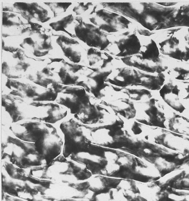
Figure 29. \{110\} surface after evaporation at 744^{\circ}\text{C} for 700 min., cylinder single crystal, oblique lighting, 1000X.
