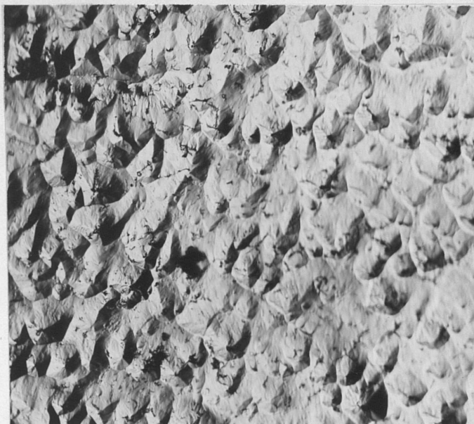
Figure 23. \{111\} surface after evaporation at 744°C for 690 min., cylinder single crystal, 200X.
