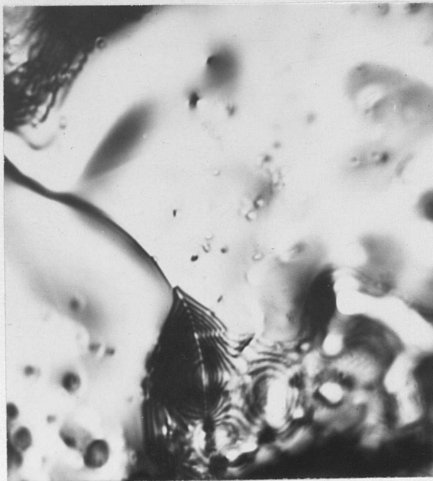
Figure 31. Grain boundary of polycrystal evaporated at 727^{\circ}\text{C} for 528 min., 1000X.
