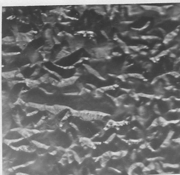
Figure 22. \{100\} surface after evaporation at 744^{\circ}\text{C} for 770 min., cylinder single crystal, oblique lighting, 1000X.
