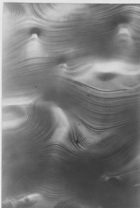
Figure 33. Ledges on chromium polycrystal, 3000X.
