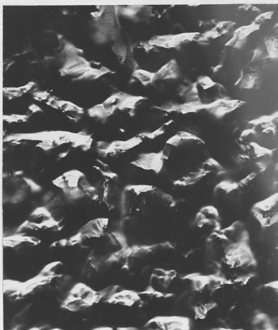
Figure 28. \{110\} surface after evaporation at 744^{\circ}\text{C} for 700 min., cylinder single crystal, 1000X.
