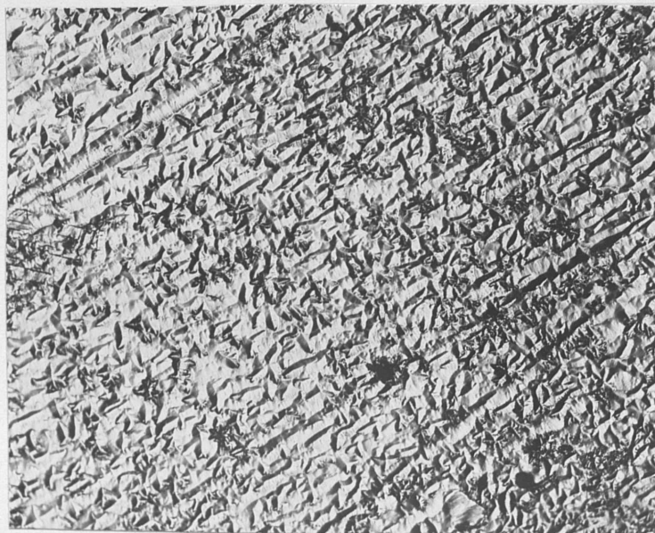
Figure 21. \{100\} surface after evaporation at 744^{\circ}\text{C} for 770 min., cylinder single crystal, 200X.
