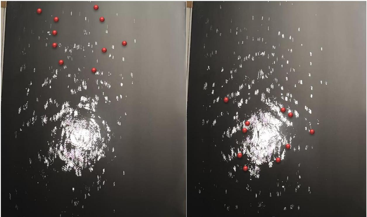
**Figure G-1 Wave Feature Tracking to Determine Average Wave Velocity for Test T457\_048**
