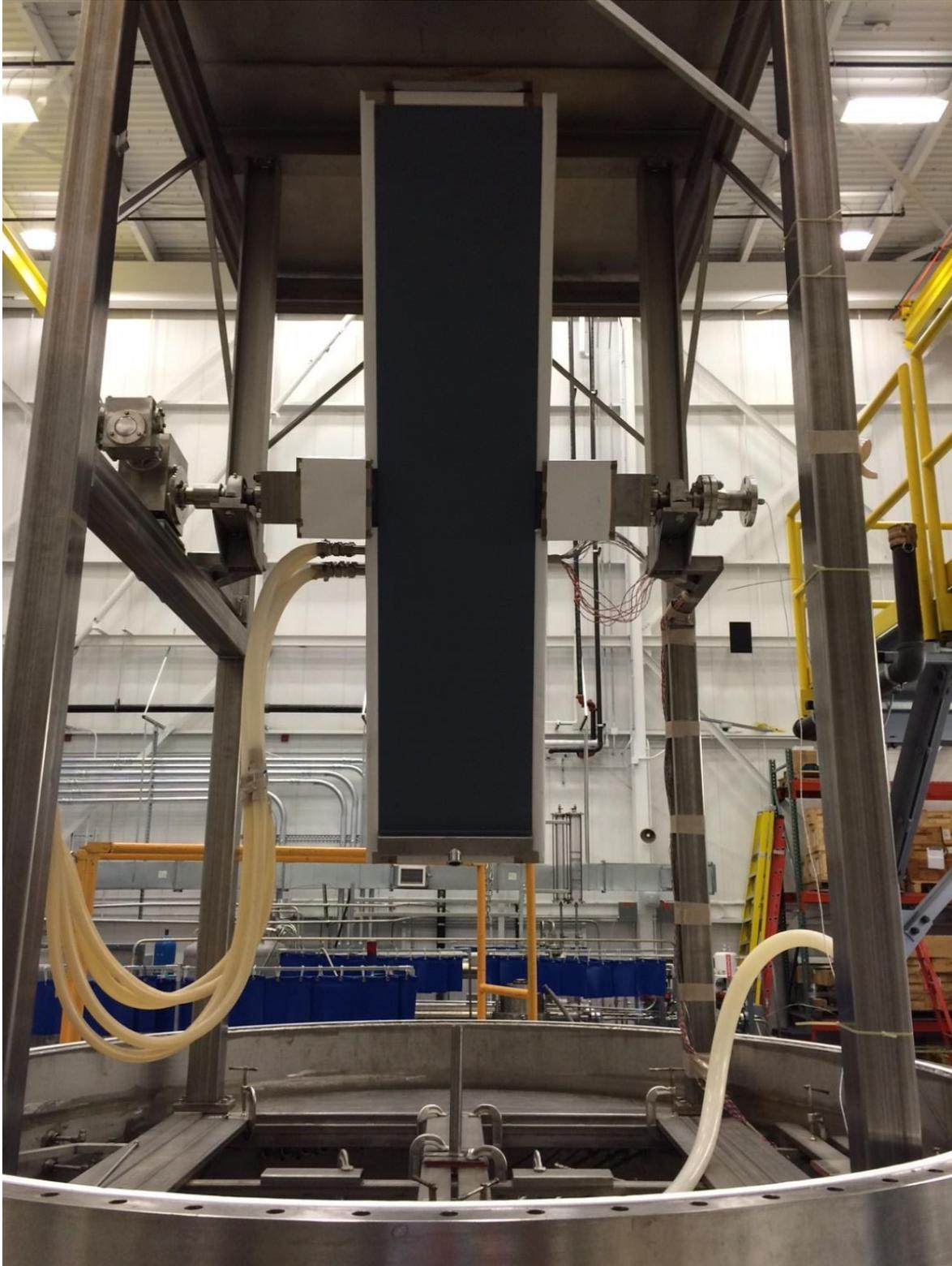
**Figure 4-9 Front Side of Test Plate Installed in Vessel with Insulation Shown on Sides**
