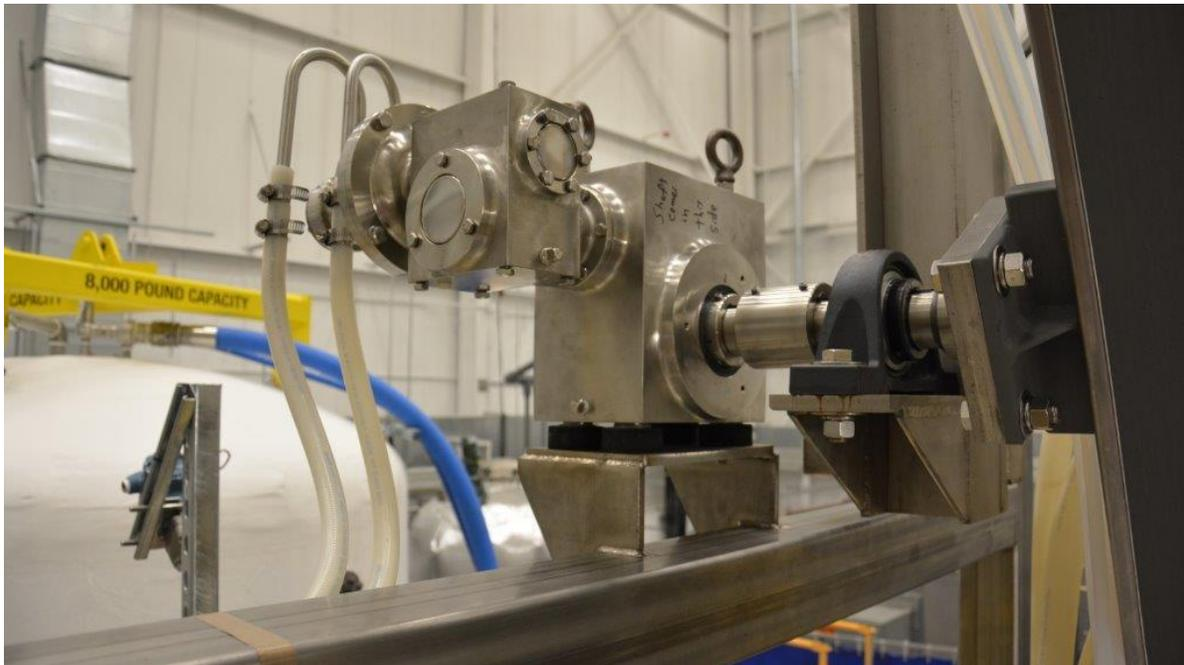
**Figure 4-4 Air Motor and Gear Box Connection with Test Plate**
