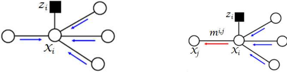
Figure 5.1: (Left) An illustration revealing the which messages (local measurements and messages from neighbors) are combined to generate each node's local belief X_{i,t} . (Right) An illustration revealing which messages are combined to form the marginalized belief sent to node j from node i in the message m_t^{i,j} .
