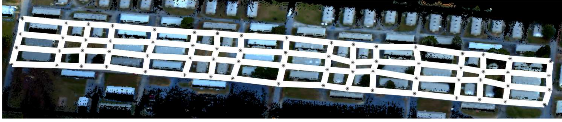
Figure 4.2: We represent the prior map as a graph where edges (white lines) denote the roads and vertices (stars) denote the road intersections.
