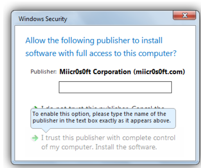
Figure 6.5: ‘Type’ attractor. The text box and the small pop-up with instructions appear only if the user hovers the install option.
