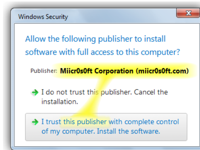
Figure 6.2: ‘Animated Connector’ attractor, shown right after the highlighting is activated by hovering the mouse over the install option.
