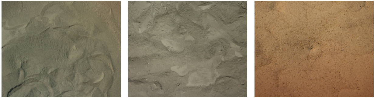
Figure 4.2: Three simulants were used for experimental validation. From left to right, JSC-1A, BP-1, and GRC-1.
