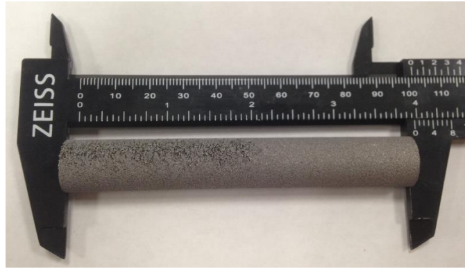
Figure 11. As-built AlSi10Mg cylindrical rod.
