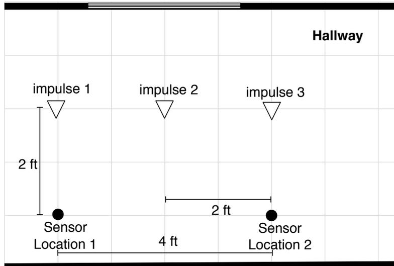
**Figure 5.23:** Ball drop experiment setting. The diagram indicates the relative locations of geophones (circles) and ball drops (triangles). The grid dimensions are  $1' \times 1'$ .
