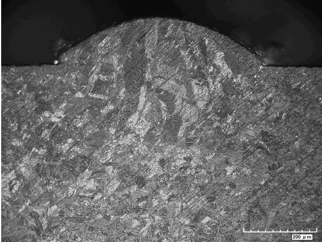
Figure 5.4: Example cross section for the electron beam powder bed process
