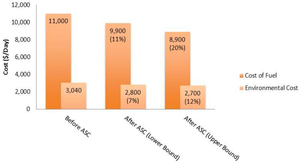
**Figure 17: Estimated Fuel and Environmental Air Emissions Cost Savings Resulting from Adaptive Signal Control System in Cranberry Township**
