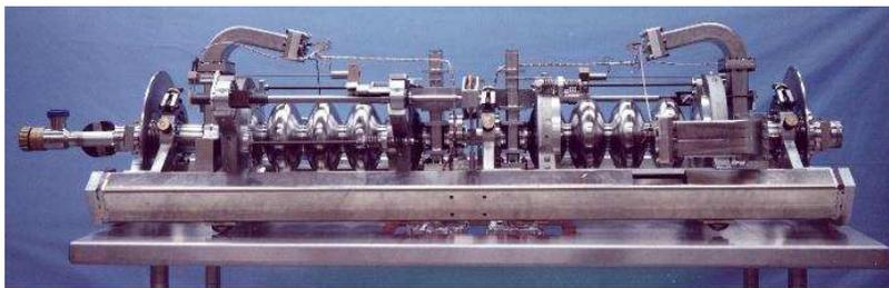
Figure 3.2: Two superconducting niobium RF cavities. In the accelerator, the cavities are located in cryomodules which use liquid helium to cool the cavities to become superconducting. From [43].
