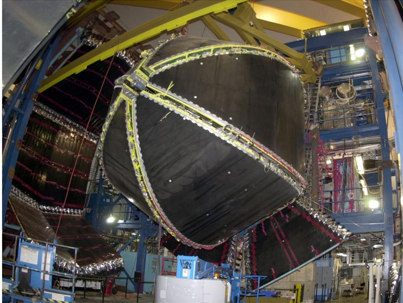
Figure 3.6: Photo of CLAS detector during maintenance, when the outer detectors (TOF scintillators, Cherenkov counters, electromagnetic calorimeters) were separated from the inner detectors. From [42].
