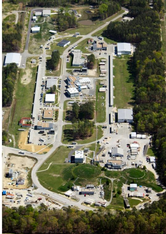
Figure 3.1: An aerial view of the Jefferson Lab site. The outline of the racetrack shaped accelerator can be seen on the surface. The three mounds of earth in the lower right cover Halls A, B, and C, from left to right. Hall D is seen in the upper left. From [42].
