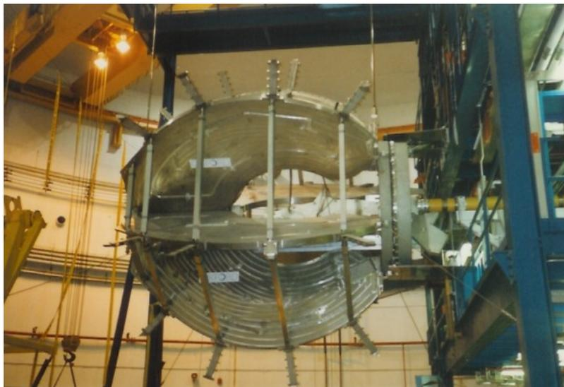
Figure 3.10: Coil cryostats of the toroidal magnet before installation of detectors. From [49].
