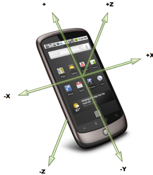
Figure 3.2: Illustration of the coordinate system of an accelerometer on a mobile phone.
