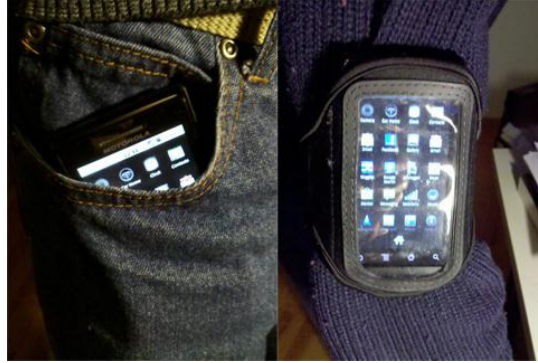
Figure 5.10: Two mounting positions of phones in experiments: stowed in pocket (left) and mounted on upper arm (right)
