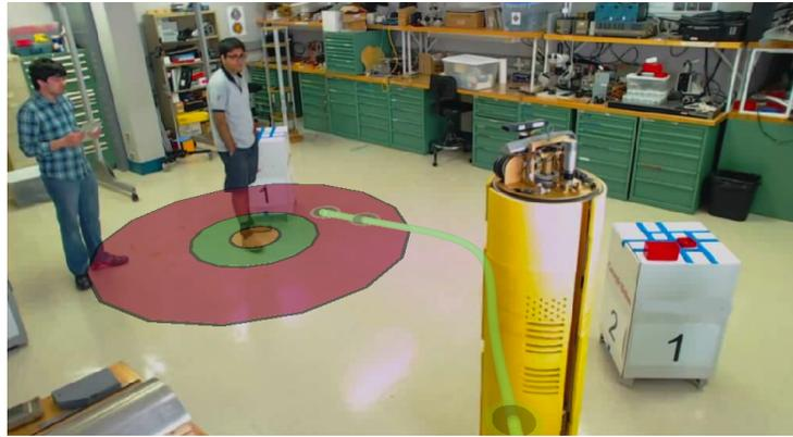
Figure 6.1: The curved trajectories planned and executed by the ballbot respect intimate and personal zones of the subject, whereas the straight line paths do not necessarily do so. Proximal zones are shown around subject: Intimate - Orange, Personal - Green, Social - Red
