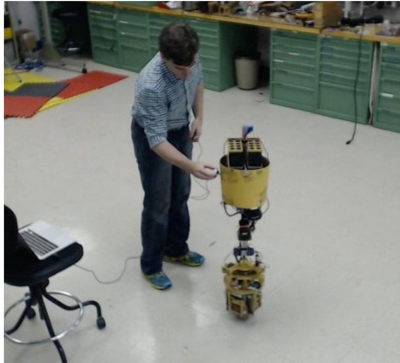
Figure 6.22: Testing force estimation with a force gauge.
