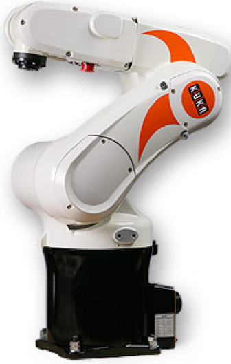
(a) KUKA KR 5 sixx R650 industrial robot
