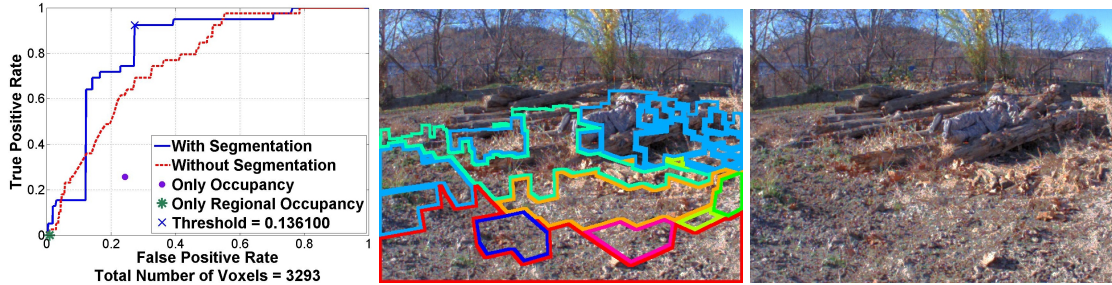
(c) In this exceptionally difficult scenario, the segmentation system was unable to distinguish camouflaged manikin from the logs resulting in a high false-positive rate before any correct changes were detected. It is possible that in this scenario the features generated for the environment are simply not rich enough to adequately characterize this scene.
