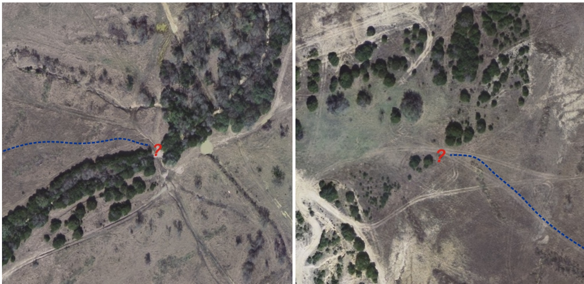
Figure 7.1: An uncertainty resolution technique that can distinguish between situations such as those above could further improve the impact of techniques such as those in this thesis. In the left image, resolving the uncertainty at this pinch point through a human query can potentially save significant time and travel distance. In the right image, the outcome of a human query cannot significantly effect the quality of the path.
