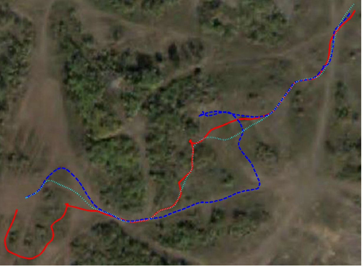
Figure 4.6: Comparison of paths executed by our robot for shown course when using only on-board perception (in solid red), and with MOLL (in dashed blue) and FROLL (in dotted cyan) used in real-time on-board the robot. Course started at the top right and ended at the bottom left.
