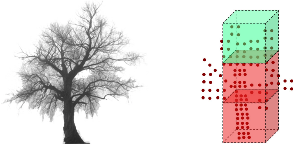
Figure 3.7: Illustration of the perception system’s voxelization of vertical columns within the environment and subsequent classification. The voxels here are actually much smaller within the system but are enlarged for demonstration purposes. In the perception system, each voxel is a 20\text{ cm}^3 cube. Due to the size of the Spinner and Crusher vehicles, 10 voxels in the vertical direction are computed at each location in order to include all potentially relevant information.
