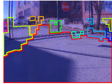
(c) \lambda = 5.0 : high smoothing parameter enforces strong segment continuity but does not allow the system to correctly segment the fence which needs to be split between more segments due to feature variation.
