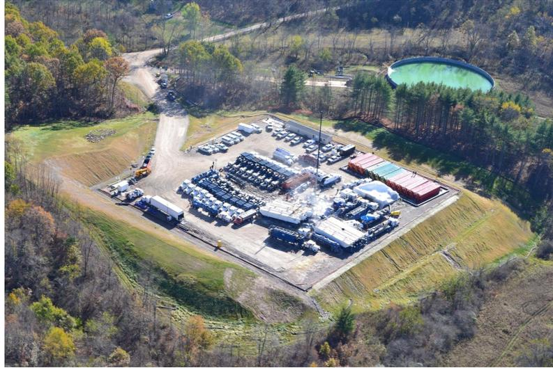
Figure 4.9: Wellpad impoundment and frac tank aerial view.
