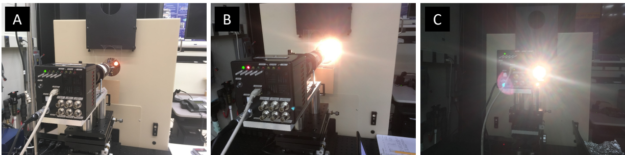
Figure 6-15: Images of successively higher temperatures emitted by the high temperature black body source at NIST. The brightness of the background changes as the images move from A to C to keep the light emitted from the black body source from saturating the image.
