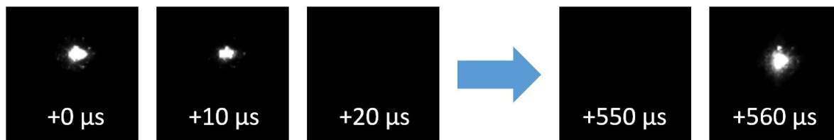
Figure 5-2: An example progression of high speed images used to determine the amount of time the beam is off for various geometries and process parameters.
