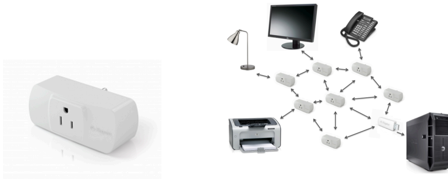
Figure 10. Plugwise circle (left) and the network between the circles and the server (right)
