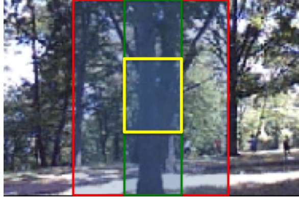
Figure 6.6: The yellow box is an example patch, the green box is the column of the same width, and the red box is the column of 3 times the patch width. Features are extracted individually at the patch, and the two columns. They are concatenated together to form the total feature representation of the patch.
