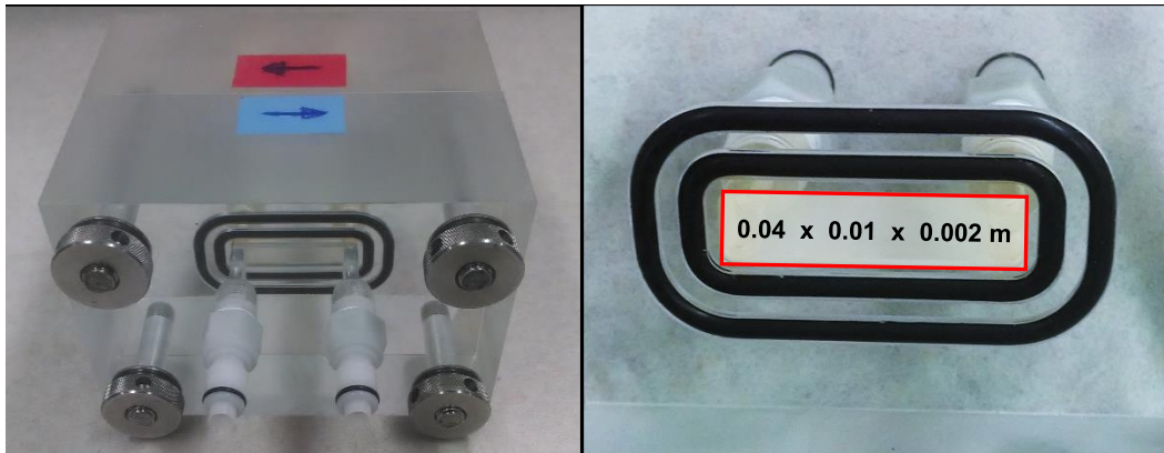
Figure C.2 Images of DCMD cassette used for data collection. Feed and permeate flow counter-current with no spacers. Channel entrance and exit are abrupt
