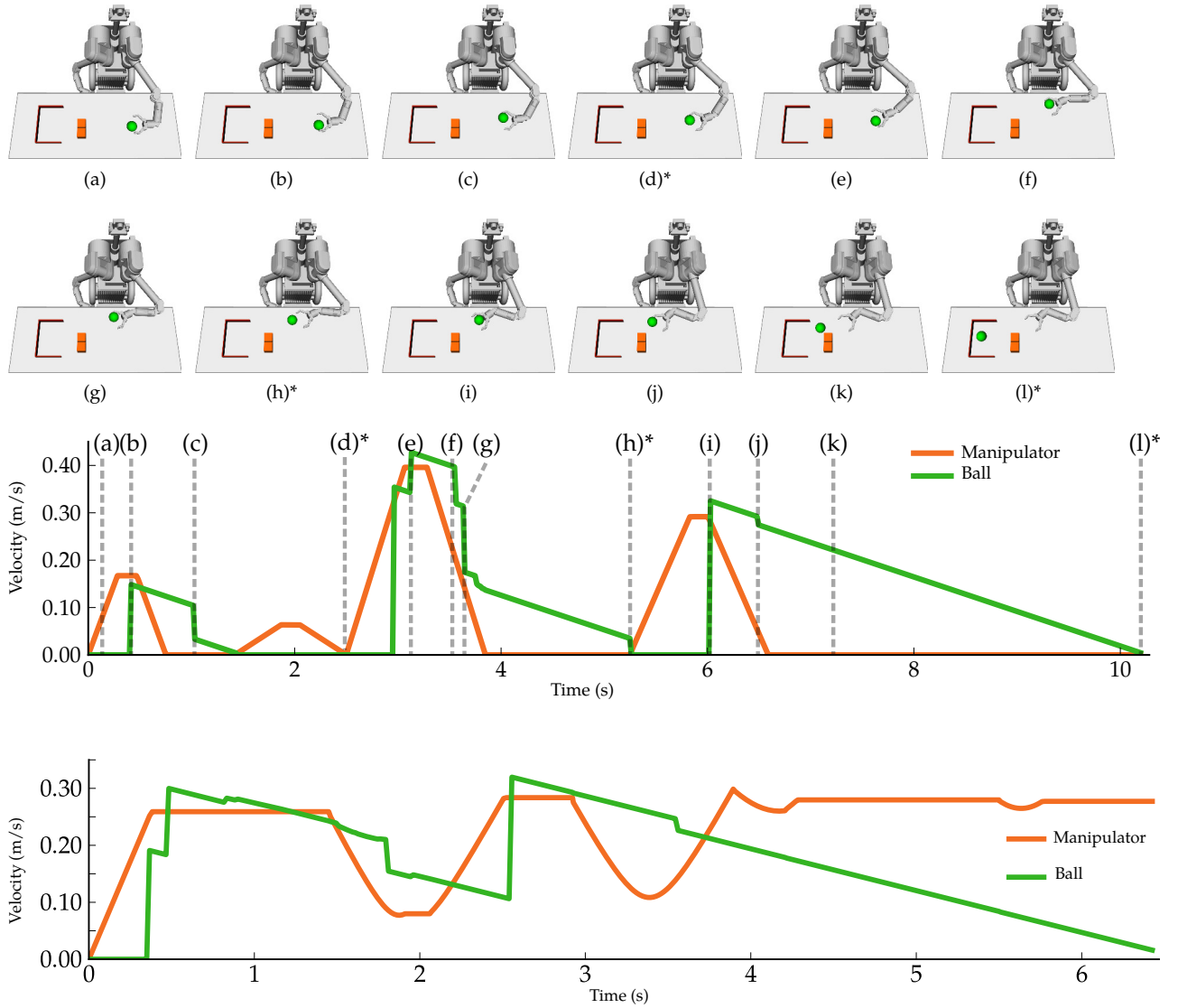
Figure 5.8: Top : Snapshots from a semi-dynamic trajectory lifted to a 7-DOF arm trajectory and executed on the robot in simulation ( T_{max} = 8s ). The task is to move the green ball into the red goal. The orange boxes are static obstacles. The states marked with * are statically stable. Middle : Velocity profile of the end-effector and the target. Note how the robot waits until the ball comes to rest before it performs the next action. Bottom : Velocities for a dynamic trajectory for the same scene. In contrast to the semi-dynamic trajectory the environment does not come to rest after each action.
