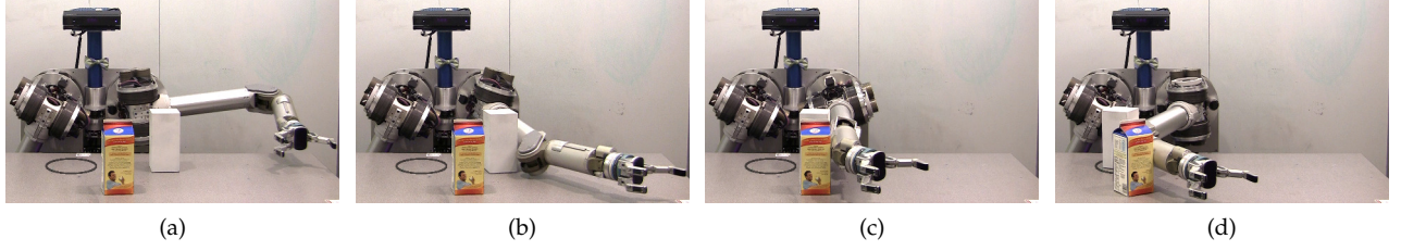
Figure 8.8: Trajectory 7, from the results presented in Fig.8.7, executed on HERB. The trajectory selection algorithm chose to use a sweeping motion to robustly push the white box into the circular goal region.
