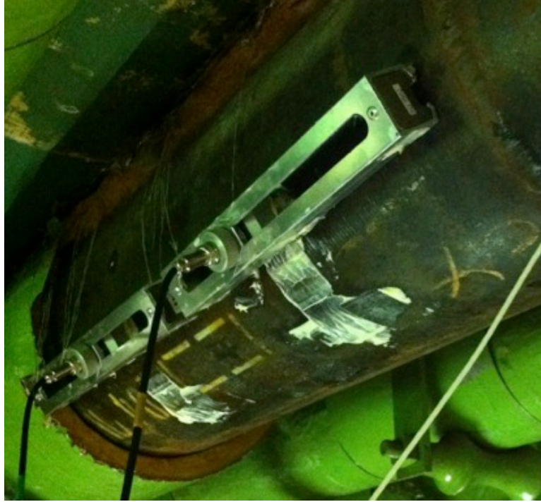
Figure 2-5 Photo of the Doppler-based flow rate gauge on the hot water pipe in field experiments
