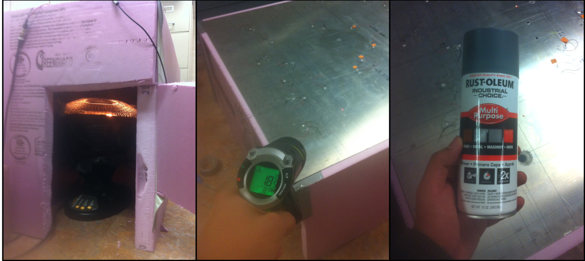
Figure 5-5 (a) A heater is placed inside the temperature chamber to heat the plate at the location indicated in Figure 5-2(a). (b) Temperature measured with hand-held laser IR thermometer at different locations during the heating. (c) A carbon black spray was applied at temperature measurement locations to reduce reflection of the aluminum surface.
