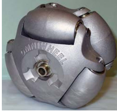
Figure 7.4: An omniwheel produced by the Kornylak Corporation. The wheel as shown is composed of two separate omniwheels, each with three rollers. Combined, the wheel can provide sideways slippage over a full 360^\circ rotation.
