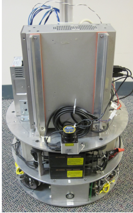
(a) Front view. Visible on the top plate are the front-mounted laser and the computer. To the left of the computer is the power supply.
