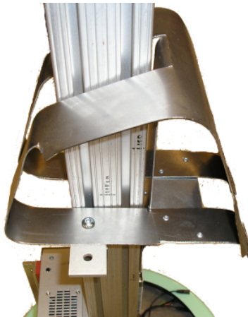
Figure 7.14: The mounting mechanism for the torso body piece is composed of a sheet-metal armature that fits onto the 80/20 pole. The mount was designed by Roni Cafri.
