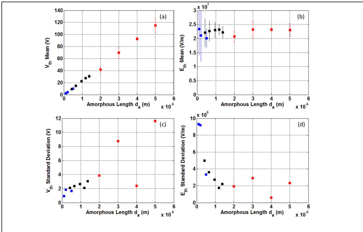
Figure 4.12 Means of (a)  $V_{th}$  and (b)  $E_{th}$  as a function of  $d_a$ . Standard deviations of (c)  $V_{th}$  and (d)  $E_{th}$  as a function of  $d_a$ . The data were measured using devices with all three different structures. Blue represents the vertical structures, black represents the lateral structures defined by E-beam and red represents the lateral structures defined by optical lithography.
