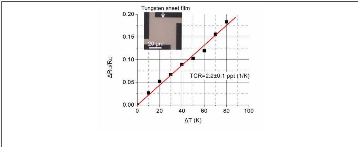
Figure 2.7 TCR measurement results. (Insert) Van der Pauw structure used to measure sheet resistance for TCR measurements.
