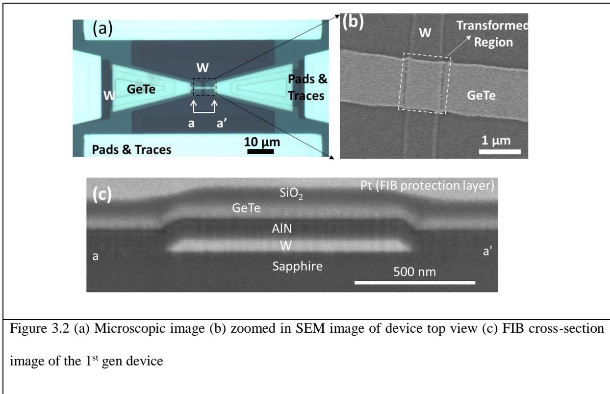
Figure 3.2(c) shows the focused ion beam (FIB) cross-section image of this device. The tungsten thickness was determined to be 50 nm. The side wall angle of the tungsten heater is approximately  $45^\circ$ , provides good side wall coverage for the layers on top of the heater. The AlN thickness was determined to be 100 nm, considering the trade-off between the efficiency to program the PC layer and the side wall
