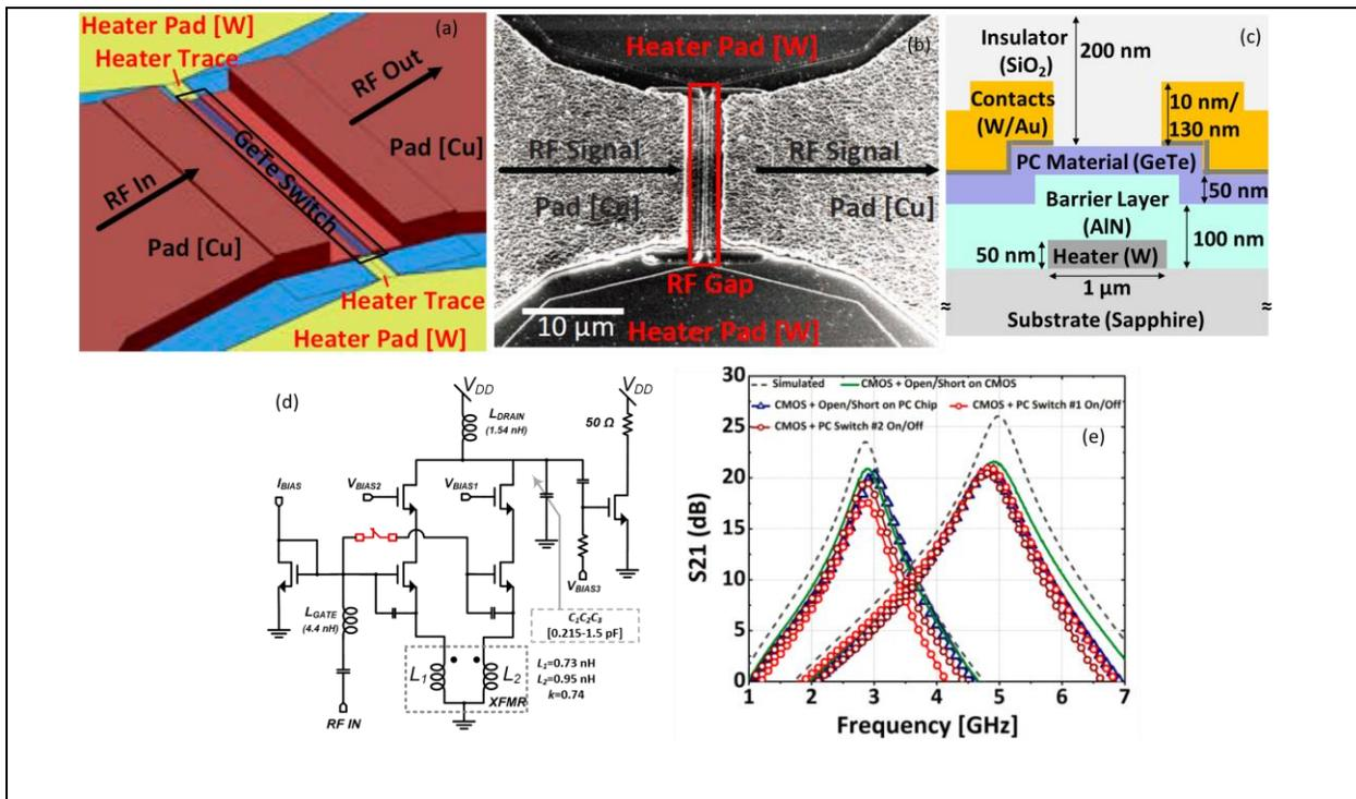
Figure 1.8. (a) 3-D perspective view (b) top view SEM image and (c) cross-section schematic of the four-terminal indirectly-heated PCS for use in the reconfigurable LNA. (d) circuit schematic of the reconfigurable LNA (e) S21 response at 3/5 GHz modes achieved by simulation, open/short on CMOS, open/short on PC chip and ON-state/OFF-state PCS. Adapted from [70] and [88].
