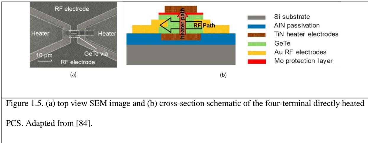
A four-terminal directly heated PCS was demonstrated by M. Wang *et al* [84]. In this architecture, as shown in Figure 1.5, two TiN heaters are vertically connected through a GeTe layer that needs to be transformed, forming the programming path. Two RF electrodes are laterally connected through the GeTe
