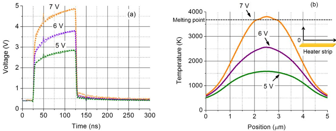
Figure 2.13 (a) Simulated (dotted lines) and experimental (solid lines) scope voltage as a function of time for different input voltages (b) Simulated temperature as a function of position at 100 ns for different input voltages
