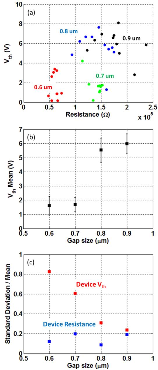
Figure 4.7 (a)  $V_{th}$  measured for RF PCS with different RF gap sizes plotted versus the OFF-state resistance of the devices (b) Mean  $V_{th}$  for the same device plotted versus the device RF gap size (c) standard deviation over mean for  $V_{th}$  (red) and OFF-state resistance (blue) versus the RF gap size
