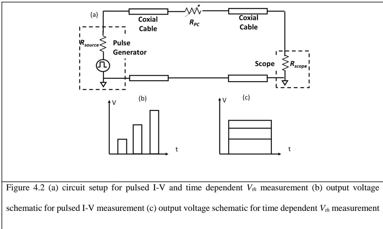
Alternatively, pulse generator can be used to generate pulsed I-V characteristic. Figure 4.2(a) shows the circuit schematic for pulse measurements on the PC devices. The pulse generator is connected with the PC device and the oscilloscope through coaxial cables and RF probes. A through setup is used so that the PC device is in series with the scope. In this way, the impedance of the scope (50  $\Omega$ ) serves as a ballast
