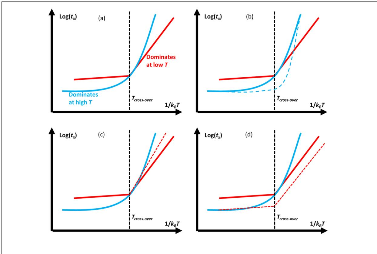
Figure 5.1 Arrhenius plot schematics for two different mechanisms controlling the crystallization at different regimes. The blue curve represents the one controlled by the free volume described by the fragility model, while the red curve represents the one independent of the free volume. Dashed curves represent the manipulations of the crystallization process to achieve either higher speed or better data retention
