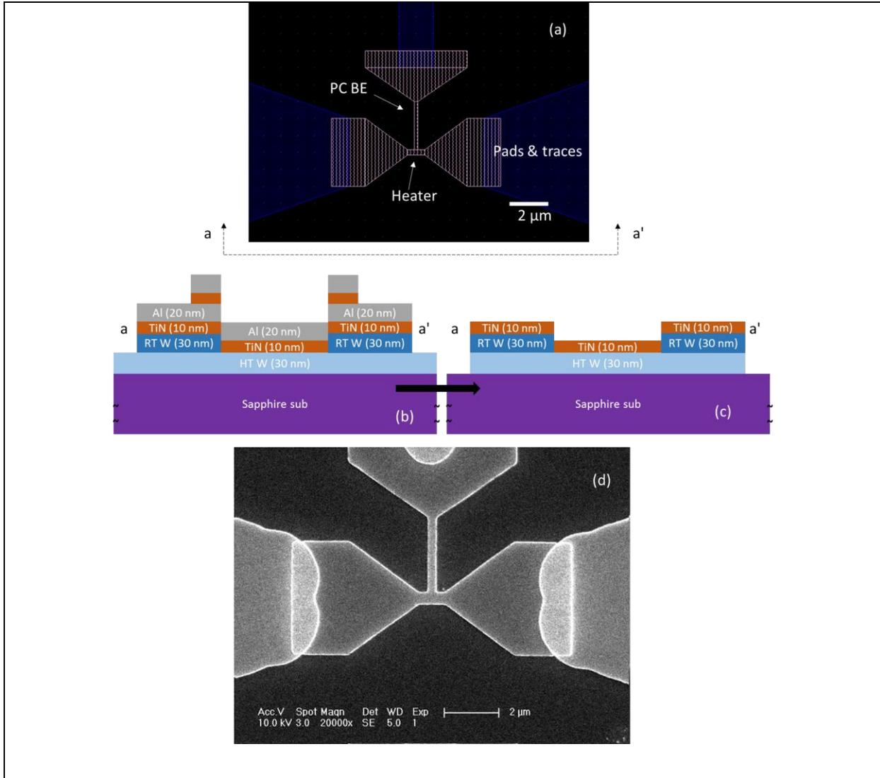
Figure 5.6 (a) layout of the first E-beam layer for patterning nano-scale heater (pink pattern) on top of the second optical layer (blue pattern). (b)-(c) process flow of patterning the HT W into the heater from cross-section view a-a'. (d) SEM image of the patterned nano-scale heater
