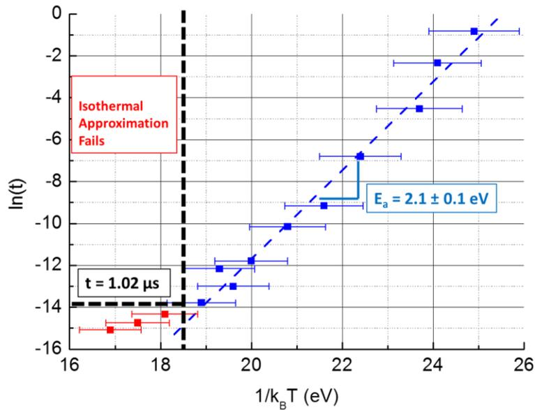
Figure 3.15 Arrhenius plot for GeTe crystallization. Blue data are used for crystallization activation energy extraction while red data are inaccurate due to the failure of the isothermal approximation. The method for correcting the non-isothermal data will be detailedly described in Chapter 7.
