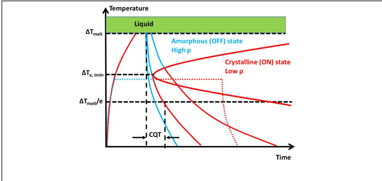
Figure 1.1. Schematic TTT diagram of PC materials and temperature transients for SET (dotted curve), successful RESET, marginal RESET and failed RESET (solid curves) operations. Red represents crystalline (ON) state for PC materials while blue represents amorphous (OFF) state.
