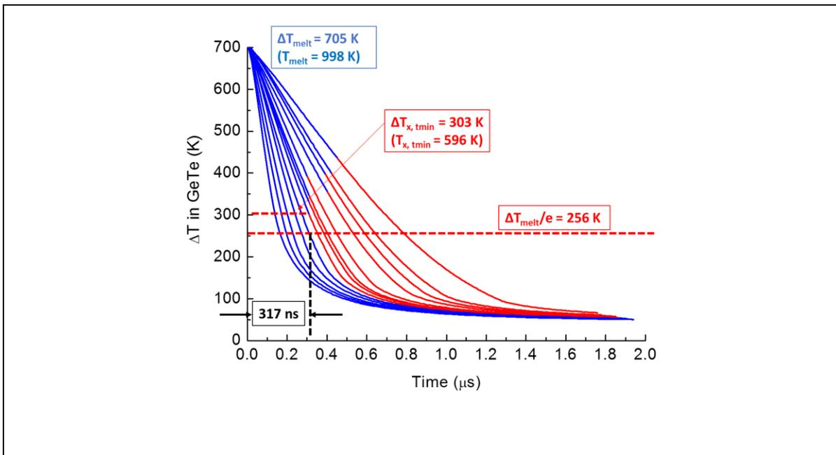
Figure 3.12 Temperature transients generated by pulses with different fall time. Blue represents OFF-state and red represents ON-state.
