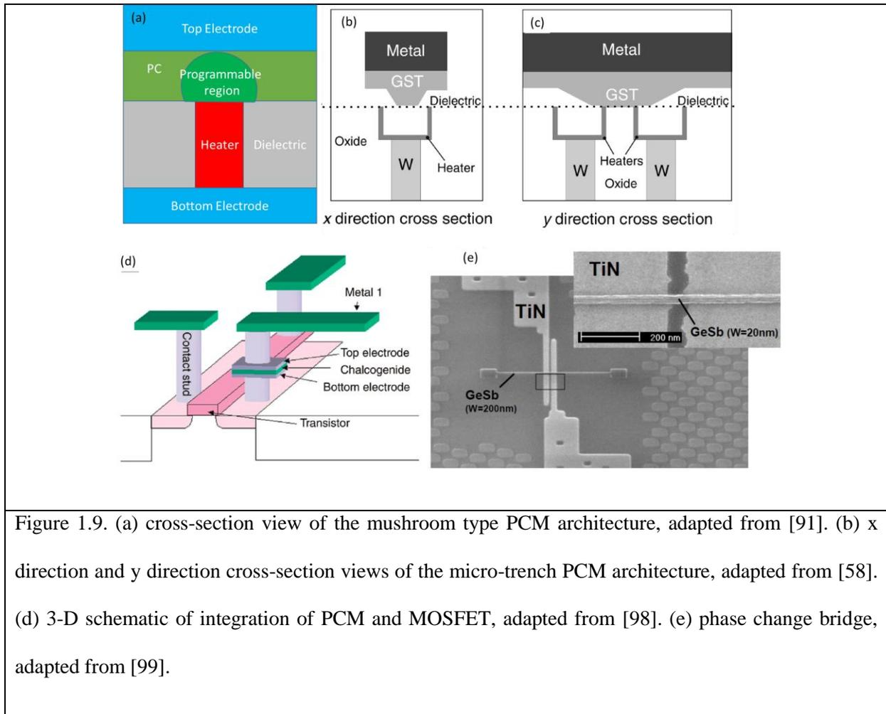
Figure 1.9. (a) cross-section view of the mushroom type PCM architecture, adapted from [91]. (b) x direction and y direction cross-section views of the micro-trench PCM architecture, adapted from [58]. (d) 3-D schematic of integration of PCM and MOSFET, adapted from [98]. (e) phase change bridge, adapted from [99].
