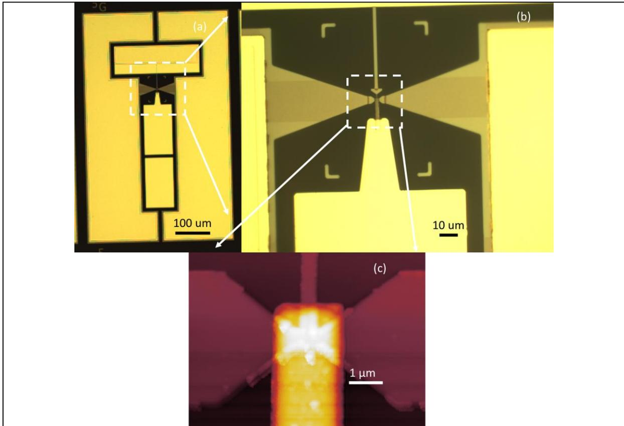
Figure 5.12 top view microscopic images of the final device (a) 1x zoomed-in view (b) 10x zoomed-in view. (c) AFM scan image of the critical section where the heater is oriented horizontally and the PC top and bottom electrodes are oriented vertically
