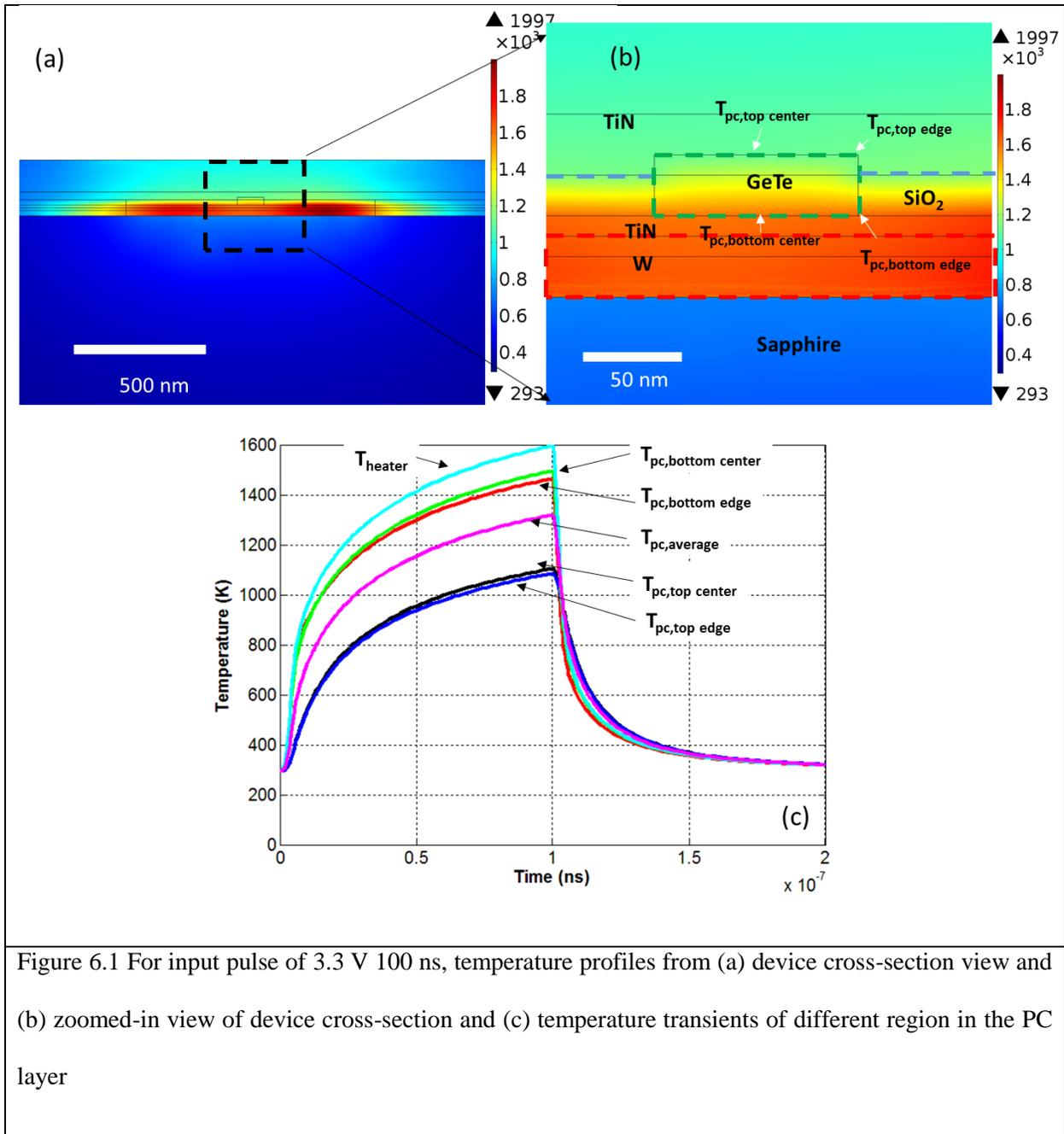
Figure 6.1 For input pulse of 3.3 V 100 ns, temperature profiles from (a) device cross-section view and (b) zoomed-in view of device cross-section and (c) temperature transients of different region in the PC layer
