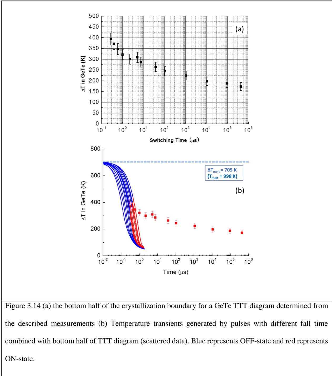
Figure 3.14 (a) the bottom half of the crystallization boundary for a GeTe TTT diagram determined from the described measurements (b) Temperature transients generated by pulses with different fall time combined with bottom half of TTT diagram (scattered data). Blue represents OFF-state and red represents ON-state.
