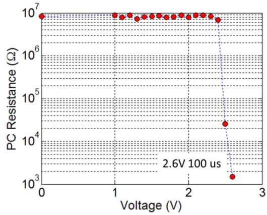
Figure 6.5 Change of PC resistance with voltage during the initial conditioning MPC process
