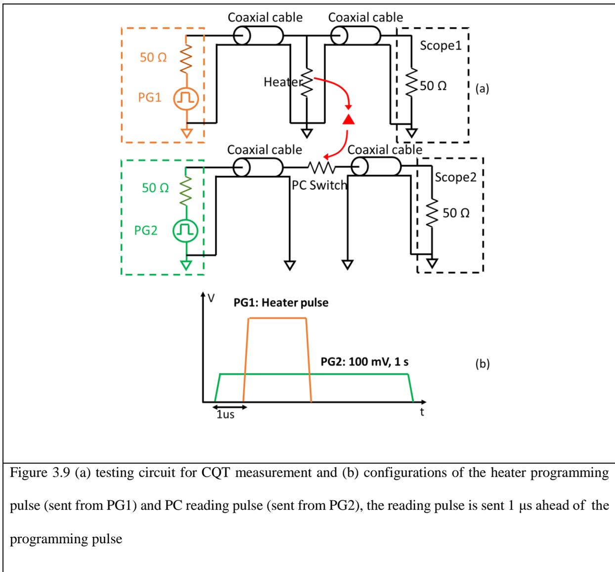
Figure 3.9 (a) testing circuit for CQT measurement and (b) configurations of the heater programming pulse (sent from PG1) and PC reading pulse (sent from PG2), the reading pulse is sent 1  $\mu$ s ahead of the programming pulse
