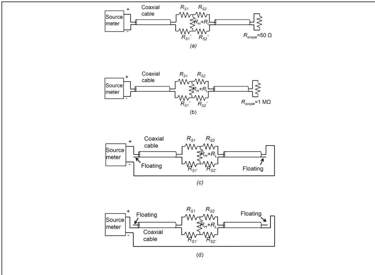
Figure 2.4 Testing circuits for parasitic resistance measurement
