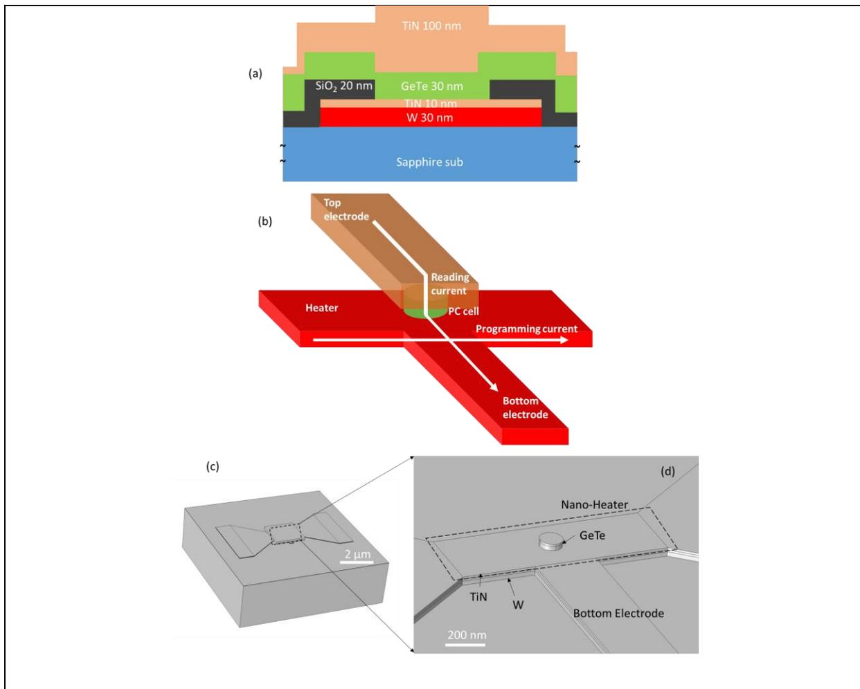
Figure 5.2 (a) cross-section and (b) 3-D perspective schematic of the 2<sup>nd</sup> gen device. (c) 3-D perspective schematic of the device structure modeled in COMSOL and (d) zoomed-in device perspective schematic with the top electrode (TiN layer) being hidden.
