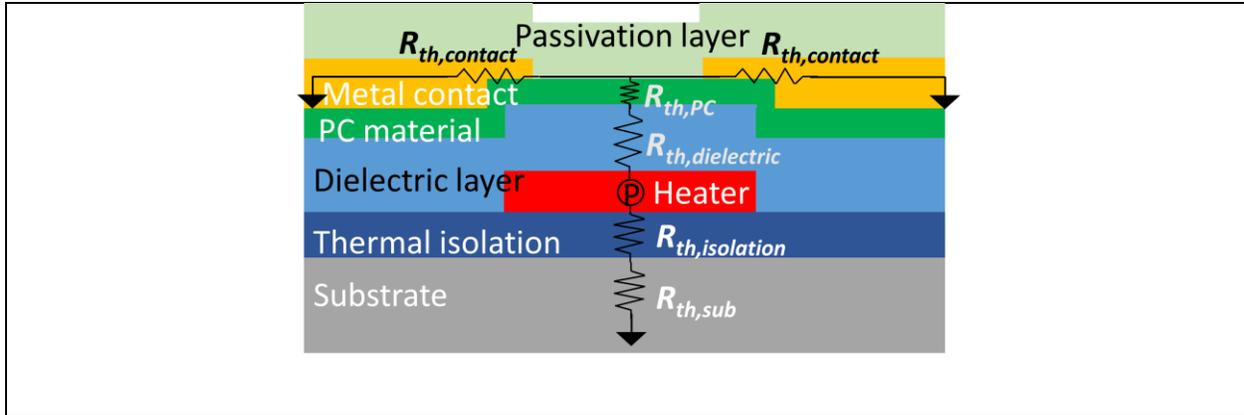
Figure 3.1. Thermal model for PCS driven by isolated heater. Thermal resistances of each layer are labeled as  $R_{th,layerName}$ .
