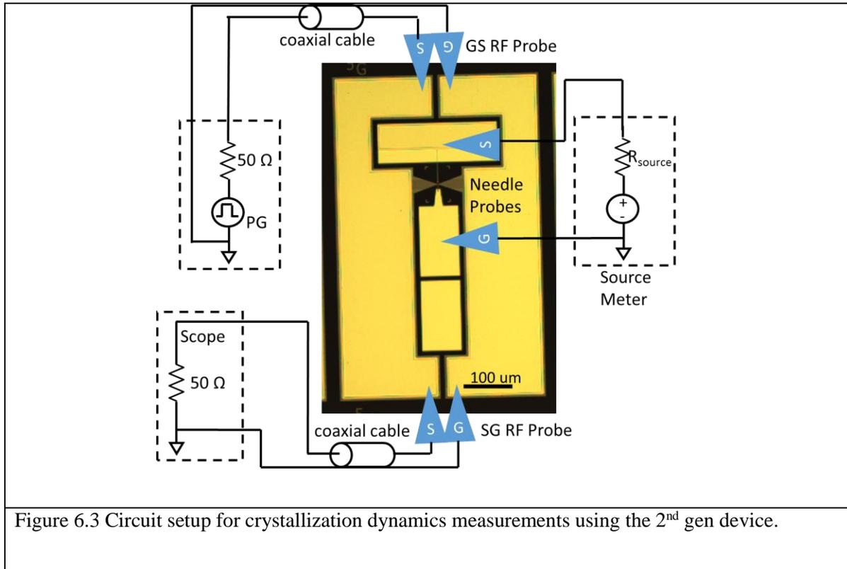
Figure 6.3 Circuit setup for crystallization dynamics measurements using the 2<sup>nd</sup> gen device.
