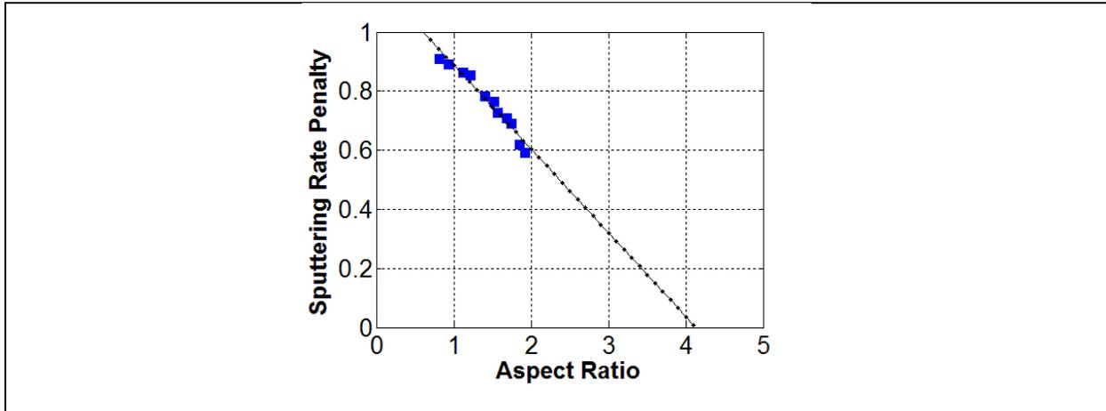
Figure 5.8 Sputtering rate penalty for the AJA sputtering system as a function of pattern aspect ratio. Blue scattered data were measured from calibration patterns, black dotted line is the fitting curve.
