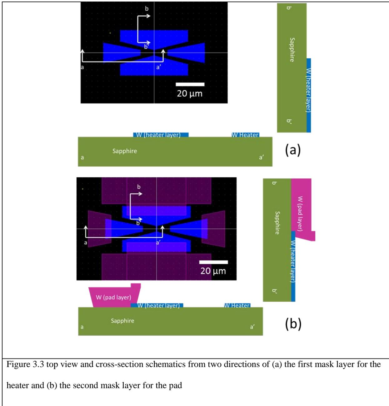
Figure 3.3 top view and cross-section schematics from two directions of (a) the first mask layer for the heater and (b) the second mask layer for the pad
