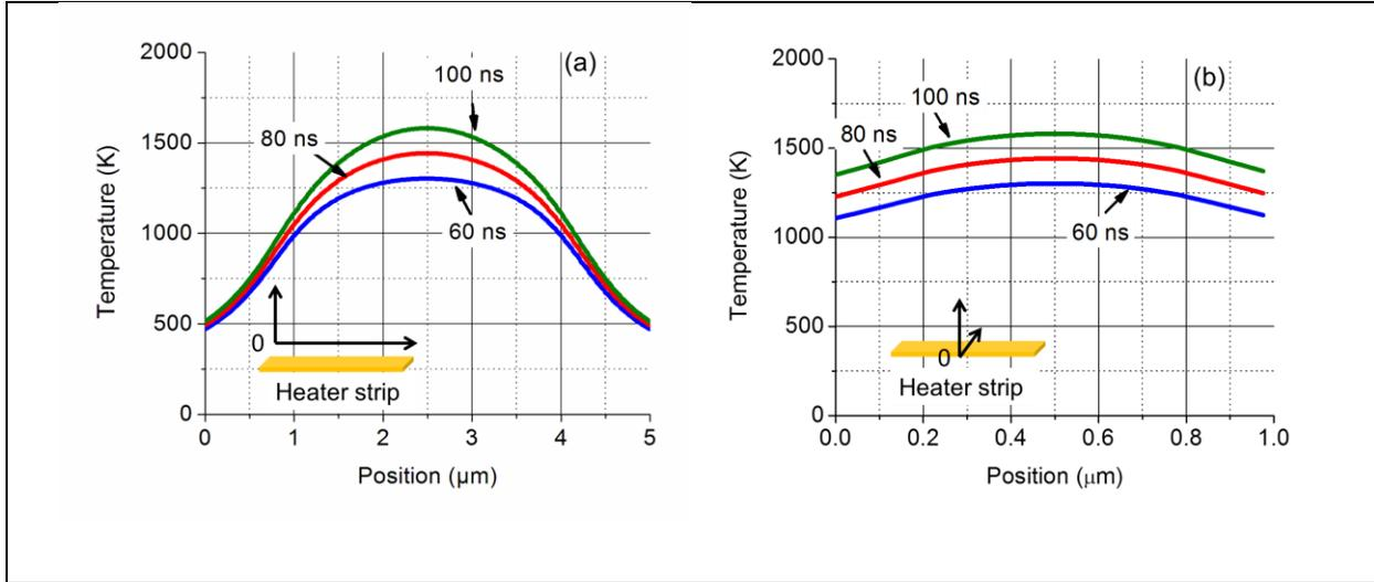
Figure 2.10 Simulated temperature profile (a) along the length of the heater and (b) along the width of the heater at 60 ns, 80 ns and 100 ns and (c) and
