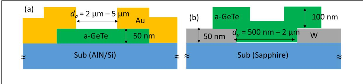
Figure 4.11 cross-section schematics for lateral amorphous structures defined by (a) optical lithography and (b) E-beam lithography
