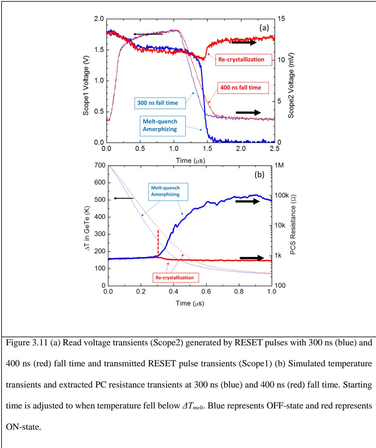
Figure 3.11 (a) Read voltage transients (Scope2) generated by RESET pulses with 300 ns (blue) and 400 ns (red) fall time and transmitted RESET pulse transients (Scope1) (b) Simulated temperature transients and extracted PC resistance transients at 300 ns (blue) and 400 ns (red) fall time. Starting time is adjusted to when temperature fell below  $\Delta T_{melt}$ . Blue represents OFF-state and red represents ON-state.
