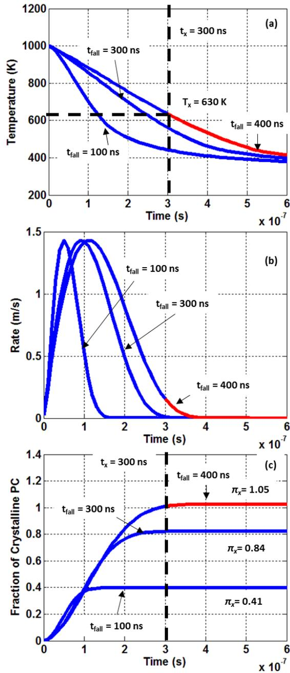
Figure 7.4 (a) temperature transients of the PC corresponding to pulse fall times  $t_{fall}$  of 100 ns, 300 ns and 400 ns, respectively. The time is adjusted to start at when the temperature just decreases below the melting point. (b) rate transients at different  $t_{fall}$  (c) transients of crystalline fraction at different  $t_{fall}$ . Blue and red color represents the PC OFF-state and ON-state respectively
