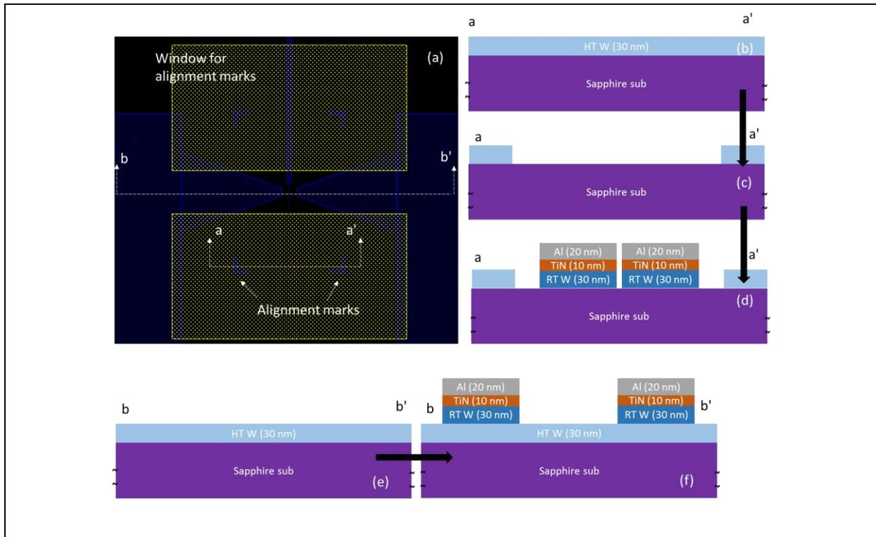
Figure 5.5 (a) the layout of the first optical mask layer for opening window through high quality tungsten (yellow dotted area) and the second optical mask layer for heater pads, traces and alignment marks. (b)-(d) and (e)-(f) show the process flow from two cross-section views of opening window through high quality tungsten, depositing and patterning alignment marks by lift-off
