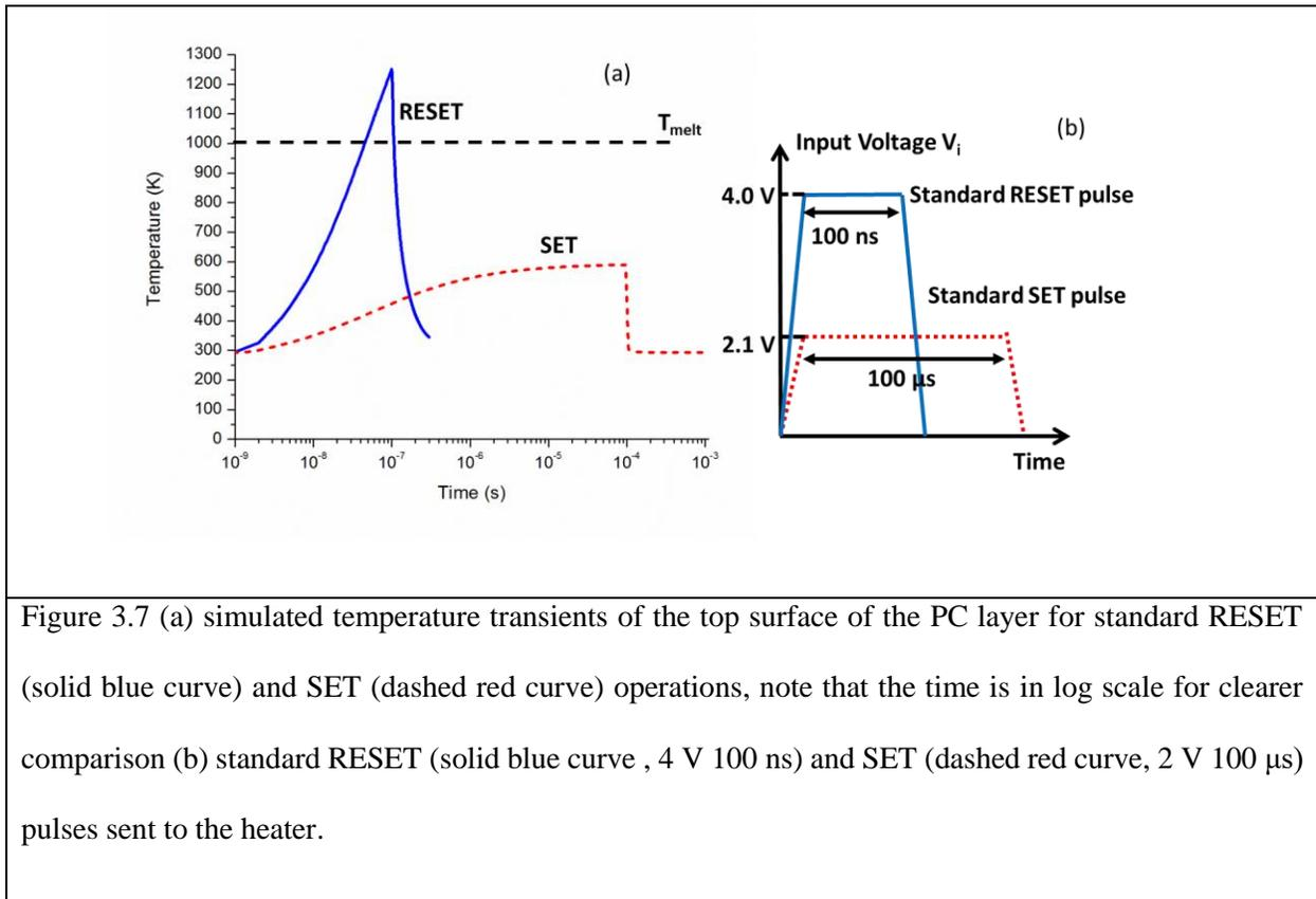
Figure 3.7 shows the simulated temperature transients based on two different electrical pulses as the heater input. The simulated transients were plotted in log scale of time for comparison between short and long transients in the same figure frame. The simulation was done using the model described in the
