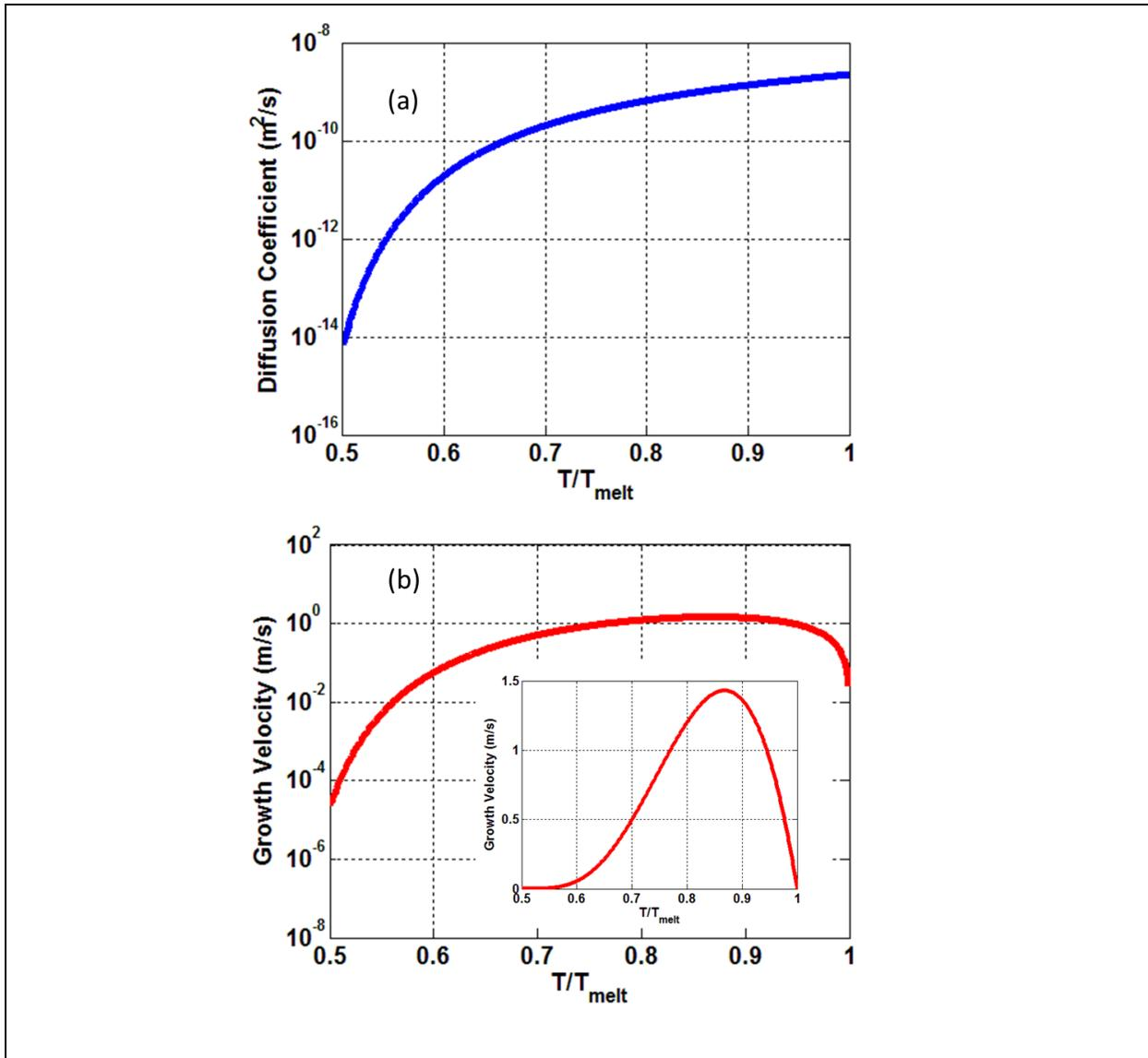
Figure 7.3 (a) diffusion coefficient  $D$  and (b) growth velocity  $v_g$  as a function of  $T/T_{melt}$ , the inset is plotted in linear scale to show maximum growth velocity
