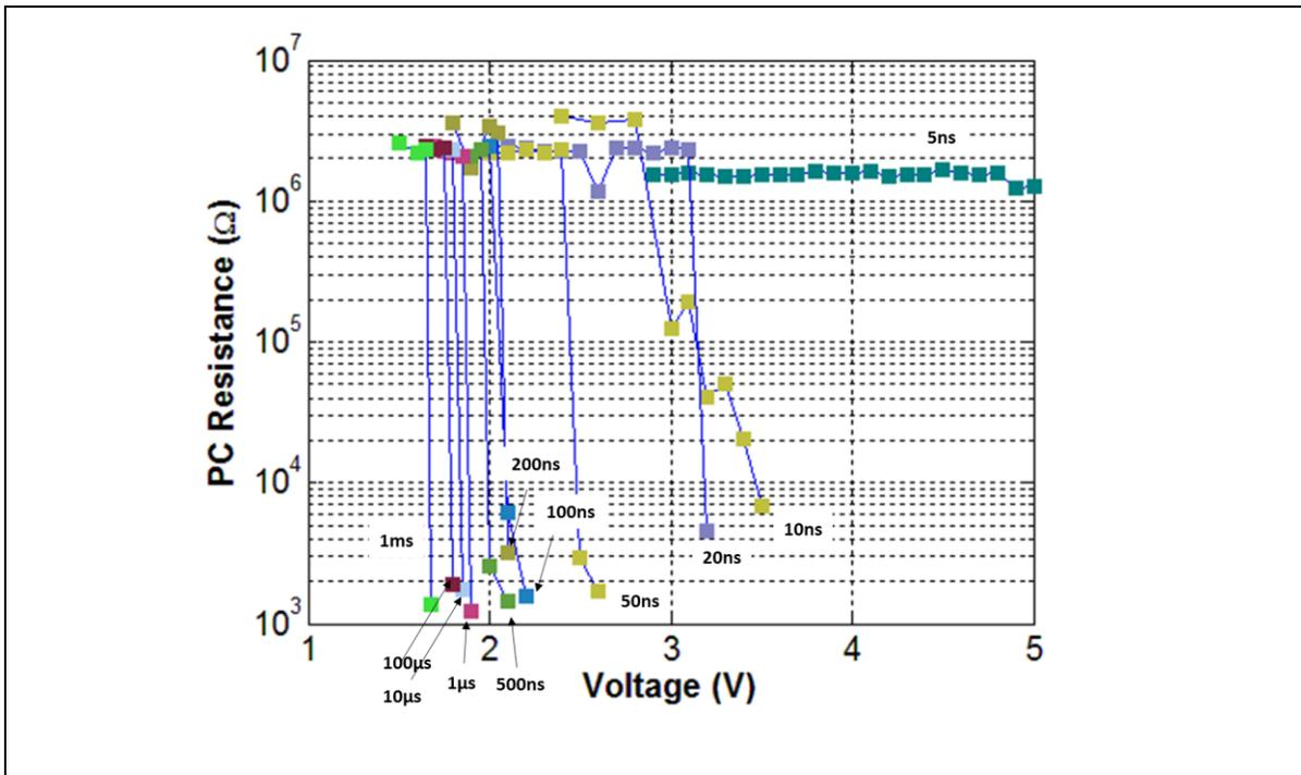
Figure 6.8 PC DC resistance measured after each crystallization pulse as a function of voltage, with different pulse widths. Note that a RESET operation is performed between each step to re-amorphize the PC layer
