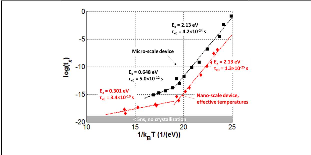
Figure 6.10 Arrhenius plot measured using the 1<sup>st</sup> gen device (black squares) and the 2<sup>nd</sup> gen device (red diamonds)
