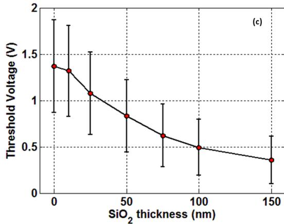
Figure 7.6 (a) simulated cross-section schematic of the temperature contour at the end of the amorphization pulse (b) estimated amorphous region sizes after each RESET and (c) estimated threshold voltage and variance as a function of SiO<sub>2</sub> thickness
