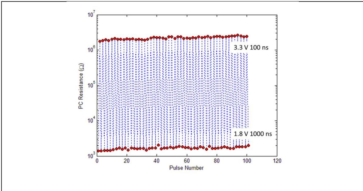
Figure 6.7 Cycleability measurement of the 2<sup>nd</sup> gen device
