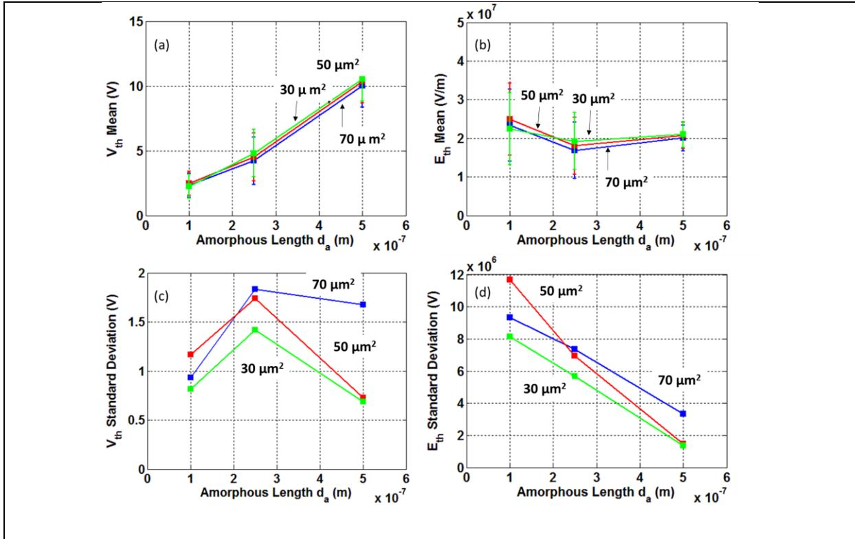
Figure 4.9 Means of (a)  $V_{th}$  and (b)  $E_{th}$  as a function of amorphous length  $d_a$ . Standard deviations of (c)  $V_{th}$  and (d)  $E_{th}$  as a function of  $d_a$
