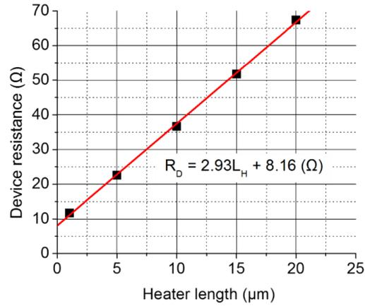
Figure 2.6 Device resistance measurements as a function of heater length, where device resistance  $R_D = R_H + R_L$
