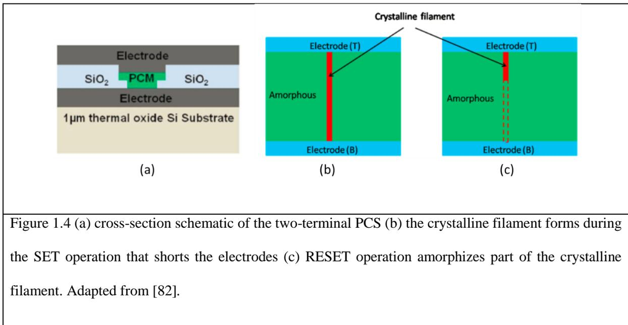
Figure 1.4 (a) cross-section schematic of the two-terminal PCS (b) the crystalline filament forms during the SET operation that shorts the electrodes (c) RESET operation amorphizes part of the crystalline filament. Adapted from [82].
