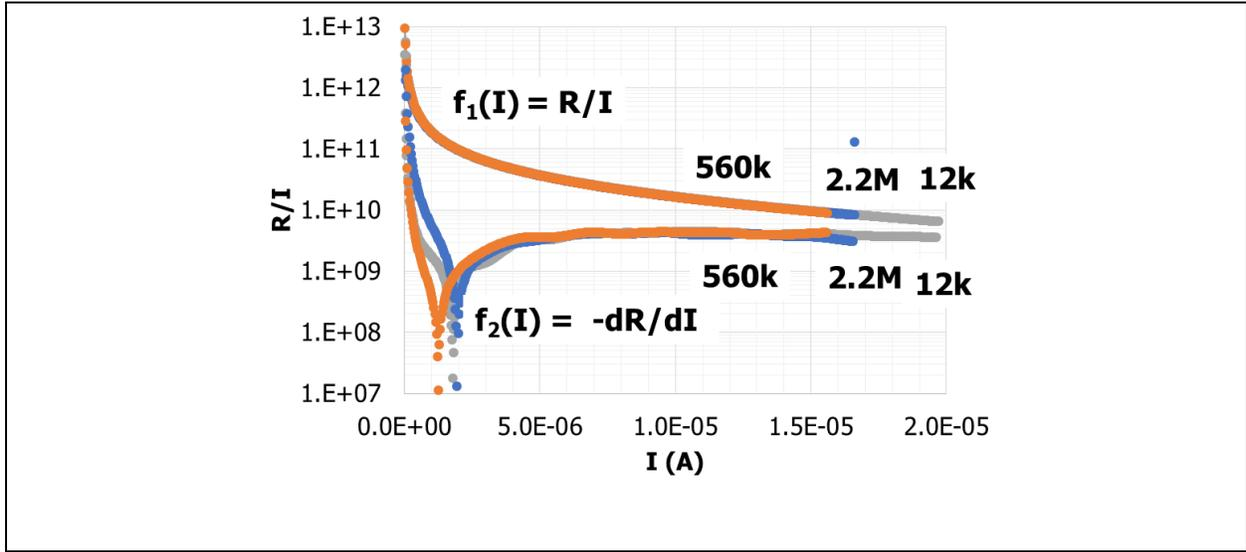
Figure 4.3 Combined plot of  $f_1(I)$  and  $f_2(I)$  for different ballast resistors
