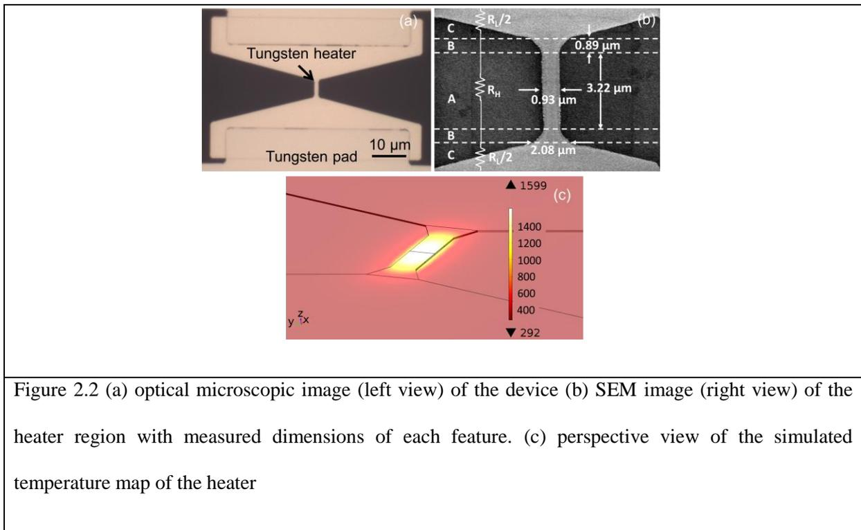
Figure 2.2 shows an optical microscope and SEM image of the heater. The central part of the heater, which is shown as part A in Figure 2.2(b), has a width of  $0.93\ \mu\text{m}$ . While the transition regions, which are
