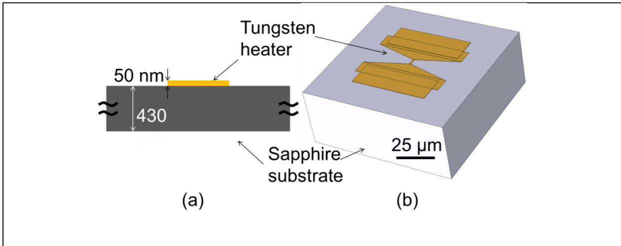
Figure 2.1 (a) cross-sectional view of the device (b) COMSOL perspective view of the device. The modeled dimensions of substrate ( $100 \mu\text{m} \times 100 \mu\text{m} \times 40 \mu\text{m}$ ) is smaller than the actual dimensions ( $25400 \mu\text{m} \times 25400 \mu\text{m} \times 430 \mu\text{m}$ ) but large enough to eliminate any substrate size effects.
