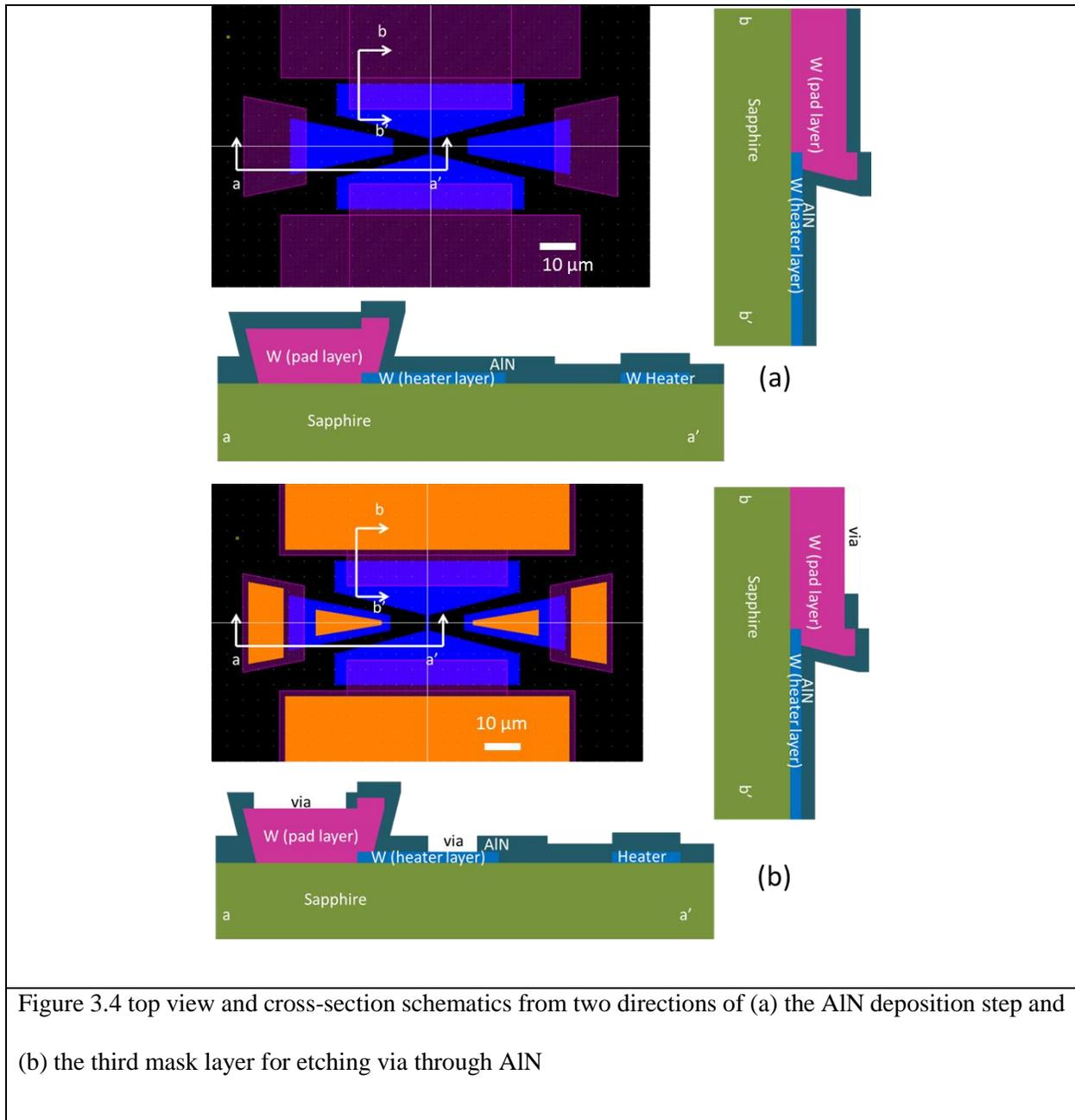
Figure 3.4 top view and cross-section schematics from two directions of (a) the AIN deposition step and (b) the third mask layer for etching via through AIN
