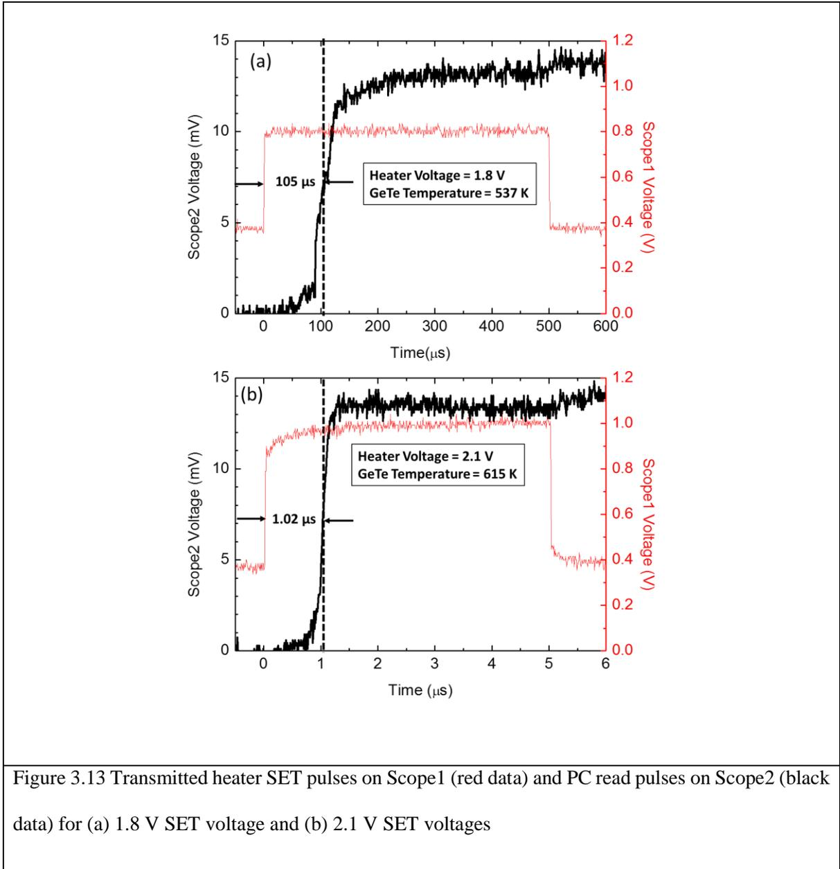
SET voltages varying from 1.6 V to 2.3 V were chosen to generate temperatures below the GeTe melting temperature for crystallization. The switching times and corresponding temperatures were measured to produce the bottom half of the crystallization boundary for the GeTe TTT diagram shown in Figure 3.14(a). Combining the bottom half of the TTT diagram with the temperature transients labelled as
