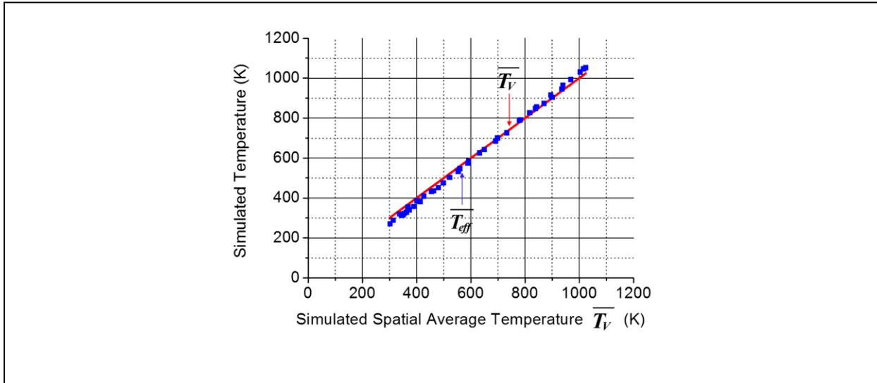
Figure 2.11 Simulated effective temperature and spatial average temperature plotted for a 5 V 100 ns pulse
