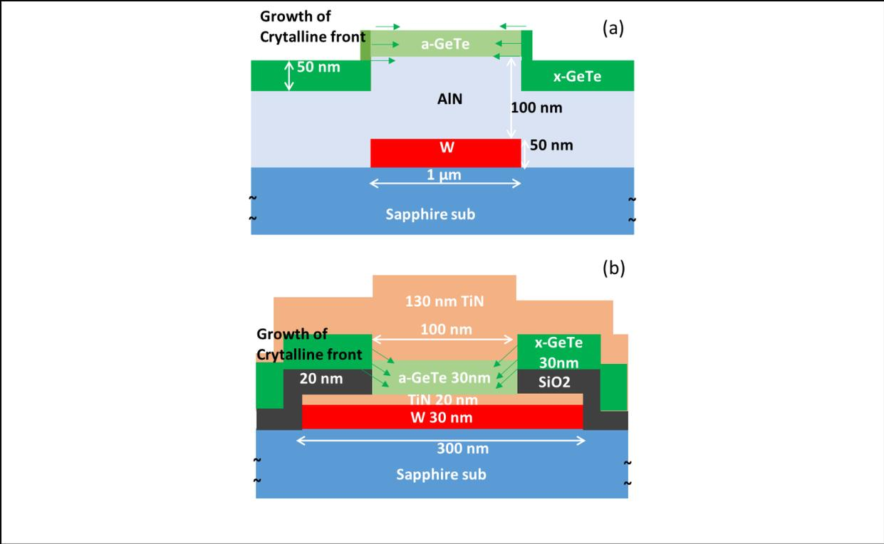
Figure 6.11 Cross-section schematics of (a) the 1<sup>st</sup> gen device and (b) the 2<sup>nd</sup> gen device. The green arrows in both figures show the direction of growth of the crystalline front during the crystallization process
