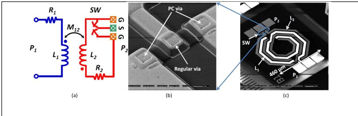
Figure 1.7. (a) circuit schematic of the reconfigurable inductor (b) SEM image of the PC via (c) SEM image of the reconfigurable inductor. Adapted from [67].
