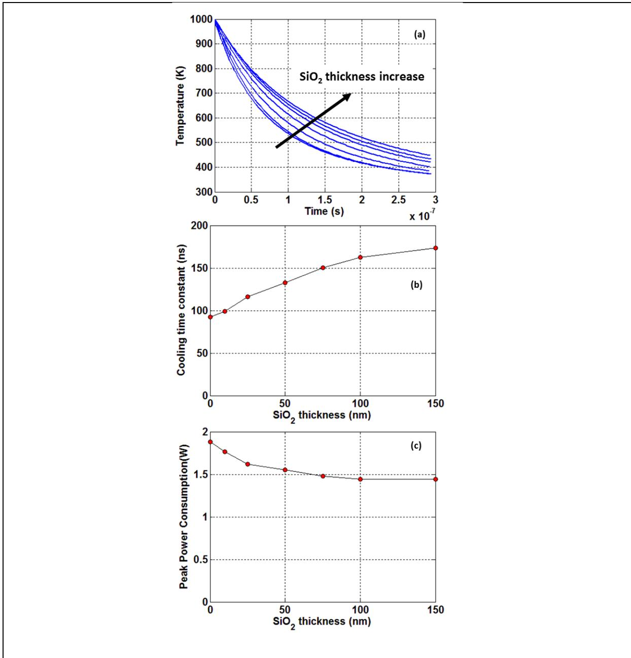
Figure 7.5 (a) temperature transients for different SiO<sub>2</sub> thicknesses, time is adjusted to start at when the temperatures just fall below the melting point (b) cooling time constant as a function of SiO<sub>2</sub> thickness (c) peak power consumption as a function of SiO<sub>2</sub> thickness
