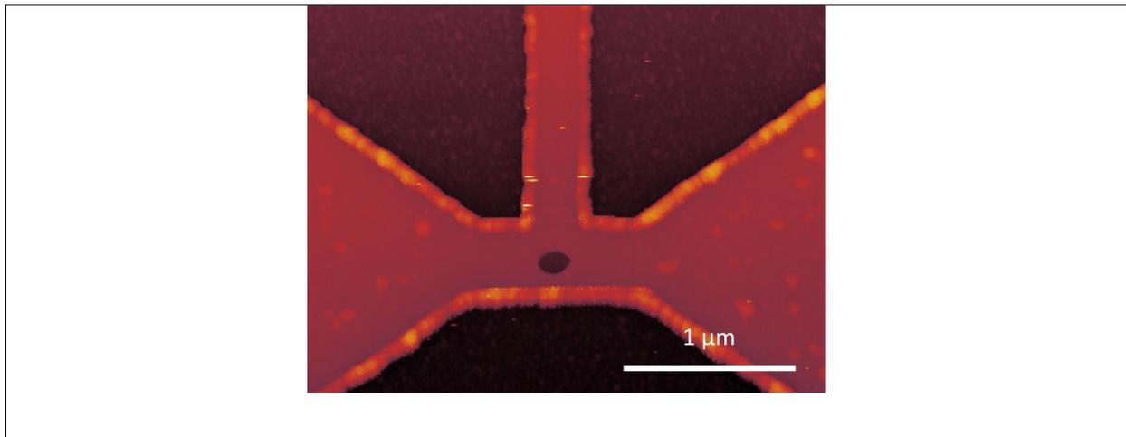
Figure 5.9 AFM scan image of the device after patterning the via through the SiO<sub>2</sub>
