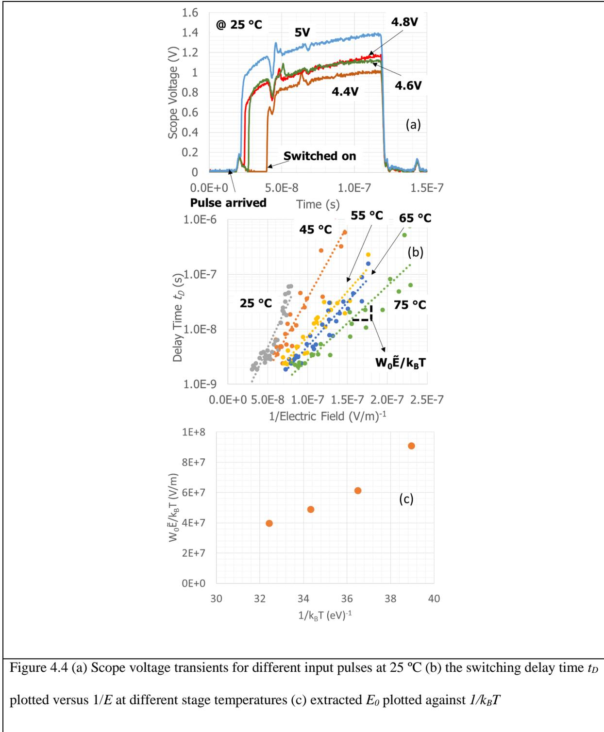
Figure 4.4 (a) Scope voltage transients for different input pulses at 25 °C (b) the switching delay time  $t_D$  plotted versus  $1/E$  at different stage temperatures (c) extracted  $E_0$  plotted against  $1/k_B T$
