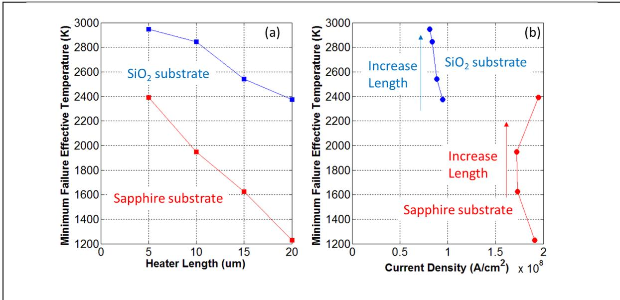
Figure 2.15 (a) minimum failure effective temperatures as a function of heater length and (b) minimum failure effective temperatures as a function of current density on sapphire substrate (red data) and SiO<sub>2</sub> substrate (blue data).
