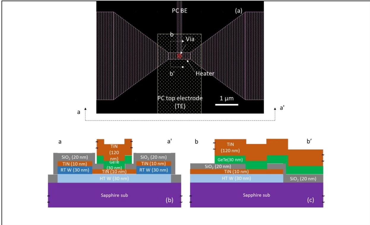
Figure 5.10 (a) the layout of the third E-beam layer for patterning PC and top electrode (yellow dashed pattern) on top of the first (pink pattern) and the second (red circle pattern) E-beam layers. (b)-(c) two cross-section views of the device after the lift-off
