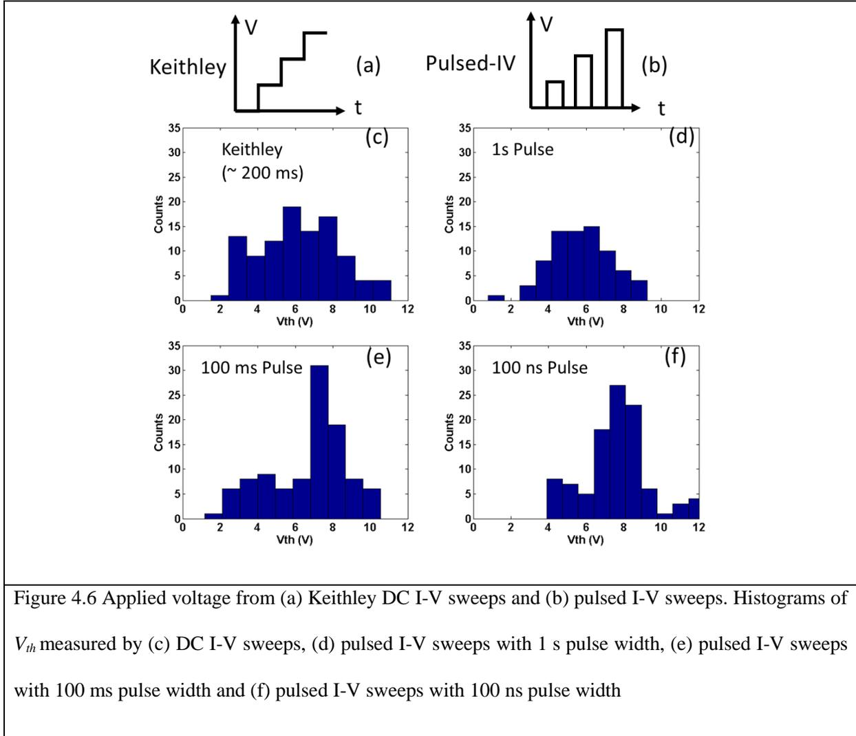
Figure 4.6 Applied voltage from (a) Keithley DC I-V sweeps and (b) pulsed I-V sweeps. Histograms of  $V_{th}$  measured by (c) DC I-V sweeps, (d) pulsed I-V sweeps with 1 s pulse width, (e) pulsed I-V sweeps with 100 ms pulse width and (f) pulsed I-V sweeps with 100 ns pulse width
