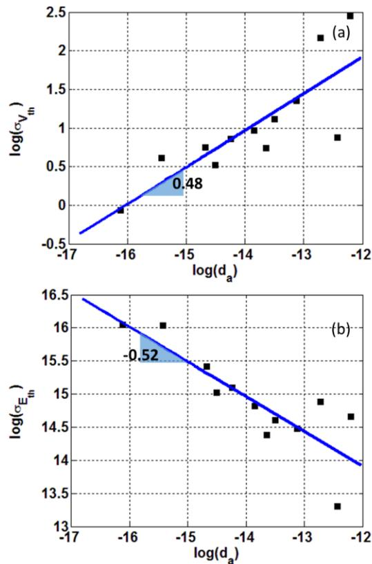
Figure 4.13 log-log plots of (a)  $V_{th}$  standard deviation versus  $d_a$  and  $E_{th}$  standard deviation versus  $d_a$
