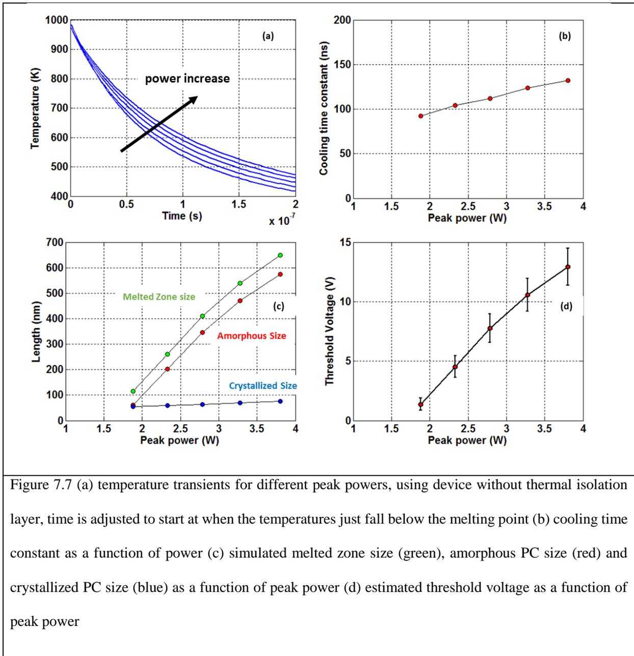
Figure 7.7 (a) temperature transients for different peak powers, using device without thermal isolation layer, time is adjusted to start at when the temperatures just fall below the melting point (b) cooling time constant as a function of power (c) simulated melted zone size (green), amorphous PC size (red) and crystallized PC size (blue) as a function of peak power (d) estimated threshold voltage as a function of peak power
