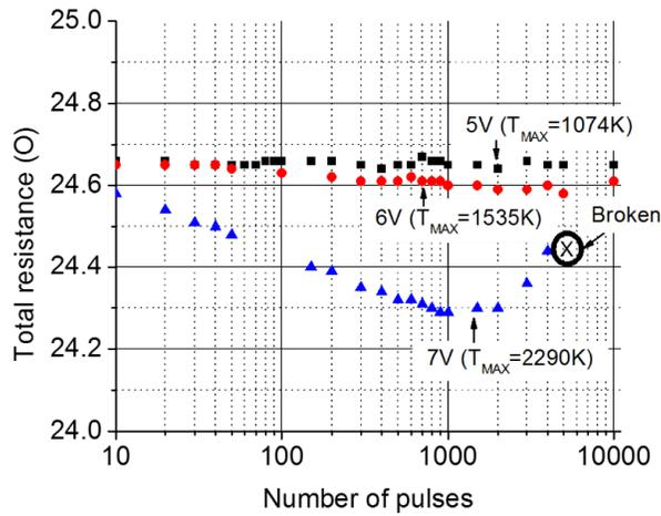
Figure 2.14 Cycling test results at different pulse height. Pulse width and pulse edge are fixed at 100 ns and 2 ns. The device was broken after 5000 pulses at 7V (maximum extracted  $\overline{T_{eff}}$  is 2290K)
