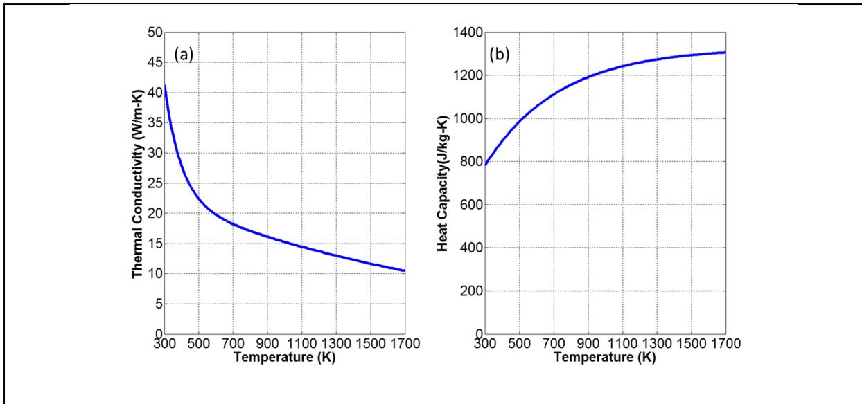
Figure 2.5 (a) temperature dependent thermal conductivity [111] and (b) temperature dependent heat capacity at constant pressure of sapphire [112]
