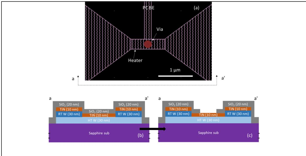
Figure 5.7 (a) layout of the second E-beam layer for via through oxide (red circle pattern in the center) on top of the first E-beam layer (pink pattern). (b)-(c) process flow of depositing SiO<sub>2</sub> and etch the via through SiO<sub>2</sub> from the cross-section view of a-a'.
