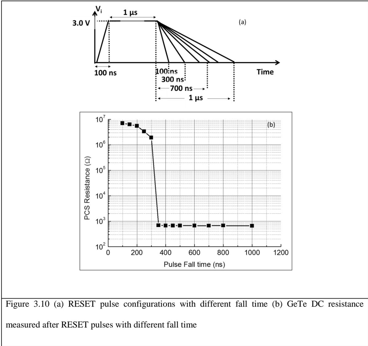
Figure 3.10 (a) RESET pulse configurations with different fall time (b) GeTe DC resistance measured after RESET pulses with different fall time
