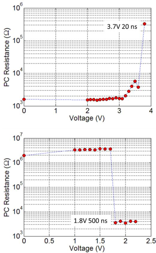
Figure 6.6 Change of PC resistance with voltage during the (a) MPA process and (b) MPC process
