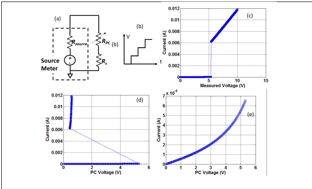
Figure 4.1 (a) DC I-V sweep circuit setup using Keithley source meter (b) schematic of source meter output voltage (c) I-V characteristic for the measured voltage and current (d) I-V characteristic for the PC device (e) zoomed in view of the PC device I-V characteristic
