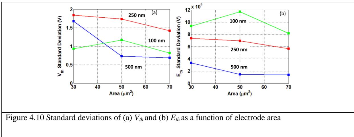
Figure 4.10 Standard deviations of (a)  $V_{th}$  and (b)  $E_{th}$  as a function of electrode area
