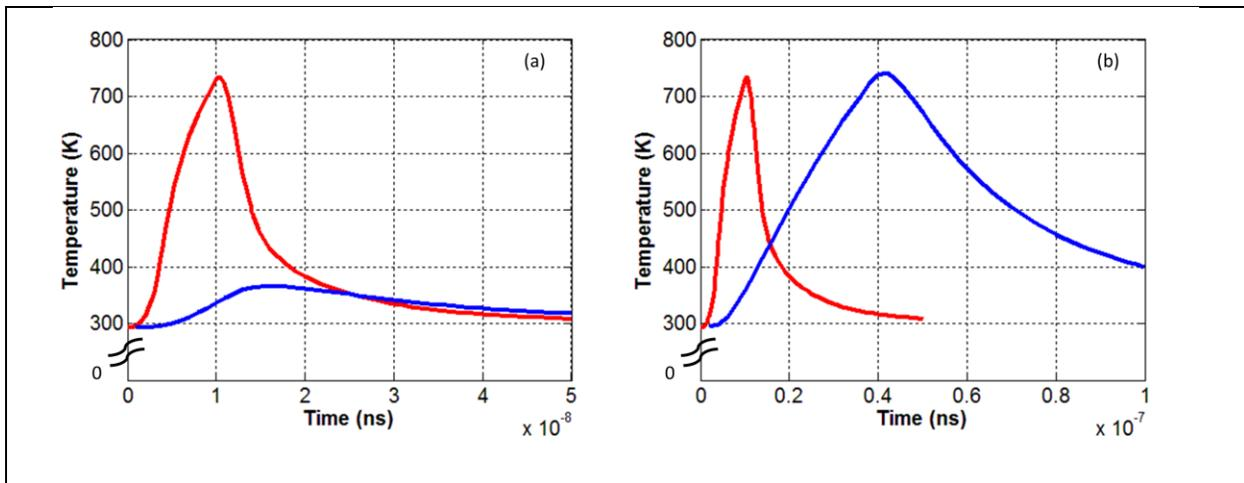
Figure 5.3 Comparison of the spatial average temperature transients in the PC layer generated by the heaters of the the 1<sup>st</sup> gen device (described in Chapter 3, blue curve) and the the 2<sup>nd</sup> gen device (red curve), (a) for the same heater pulse (3.4 V 10 ns) and (b) for the same heater voltage (3.4 V) to reach the same peak temperature
