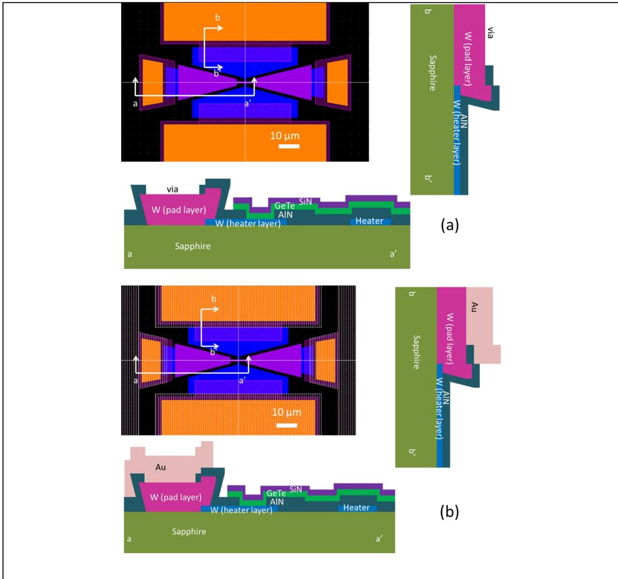
Figure 3.5 top view and cross-section schematics from two directions of (a) the fourth mask layer for PCS and (b) the fifth mask layer for metal traces
