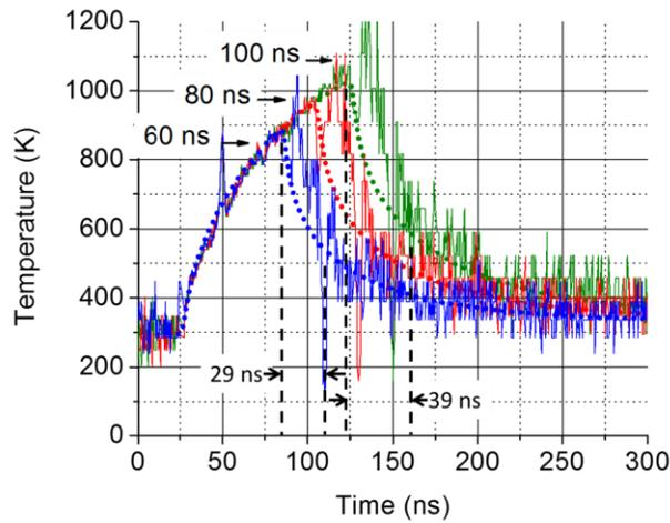
Figure 2.12 (dotted lines) simulated  $\overline{T_V}$  and (solid lines) extracted  $\overline{T_{eff}}$  according to lumped heater resistance change in Fig. 7(c) and TCR of tungsten
