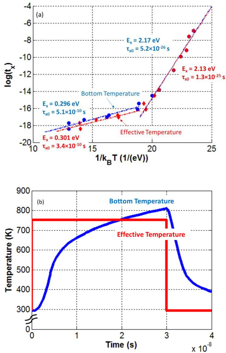
Figure 6.9 (a) Arrhenius plot generated using peak temperature at the bottom of the PC (blue) and effective temperature of the PC (red) (b) simulated temperature transient (blue) for crystallization pulse of 2.8 V 30 ns and the corresponding effective temperature transient (red)
