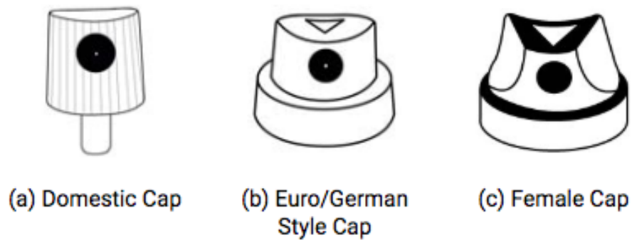
Fig.26: Types of spray can replacement nozzles [62]
